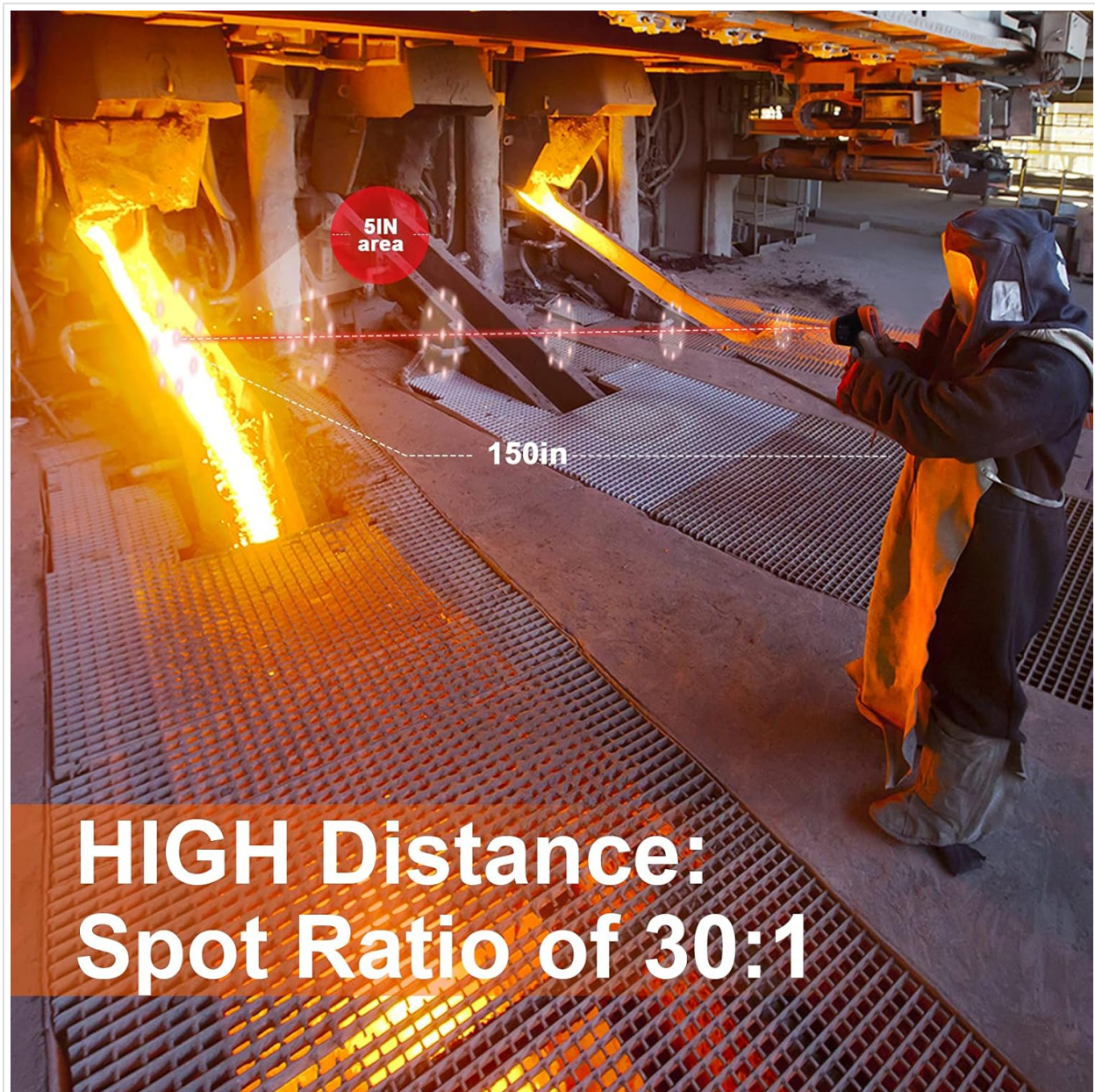
Figure 7: Illustration of the 30:1 Distance to Spot ratio, showing how the measurement area expands with distance from the target.
