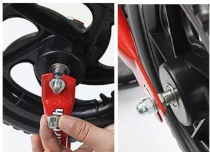
8. Install the blind nuts and tighten them. Install the second wheel in the same way
