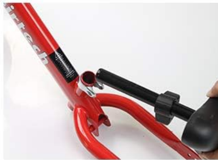
5. Install the seat post into the frame.
