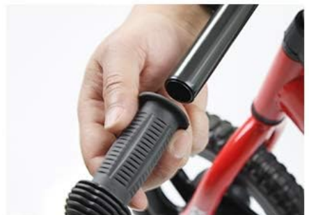
9. Place the rubber handle on top steering wheel.
