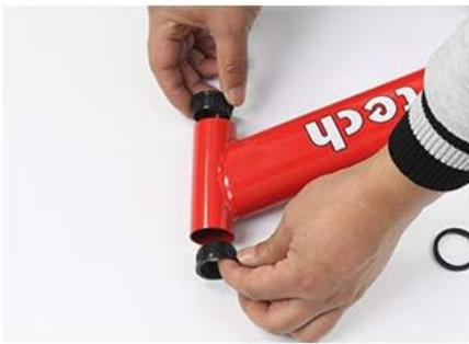
1. Prepare two large plastic sleeves and place them on the frame.
