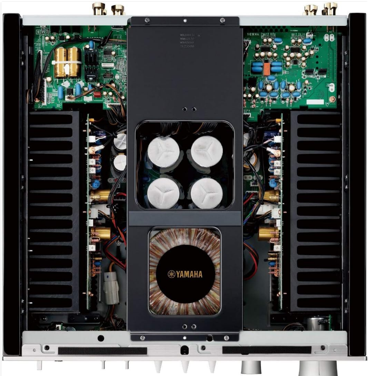
Figure 3: Internal view highlighting the toroidal power transformer and large capacitors, contributing to the amplifier's performance.
