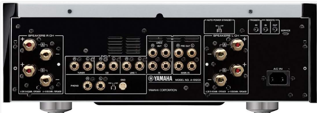
Figure 4: Rear panel connections, including speaker terminals, various audio inputs (CD, Tuner, Line 1, Line 2, Phono), and power input.
