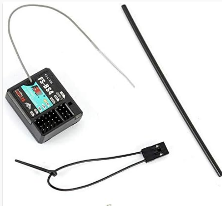
Image 4.1: The Flysky FS-BS4 receiver shown with its antenna and a bind plug, which is used during the binding process.
