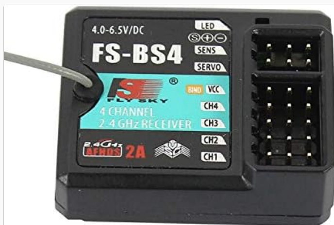
Image 2.1: Front view of the Flysky FS-BS4 receiver, showing the LED indicator, SENS and SERVO adjustment ports, BIND/VCC port, and channels CH1-CH4.
