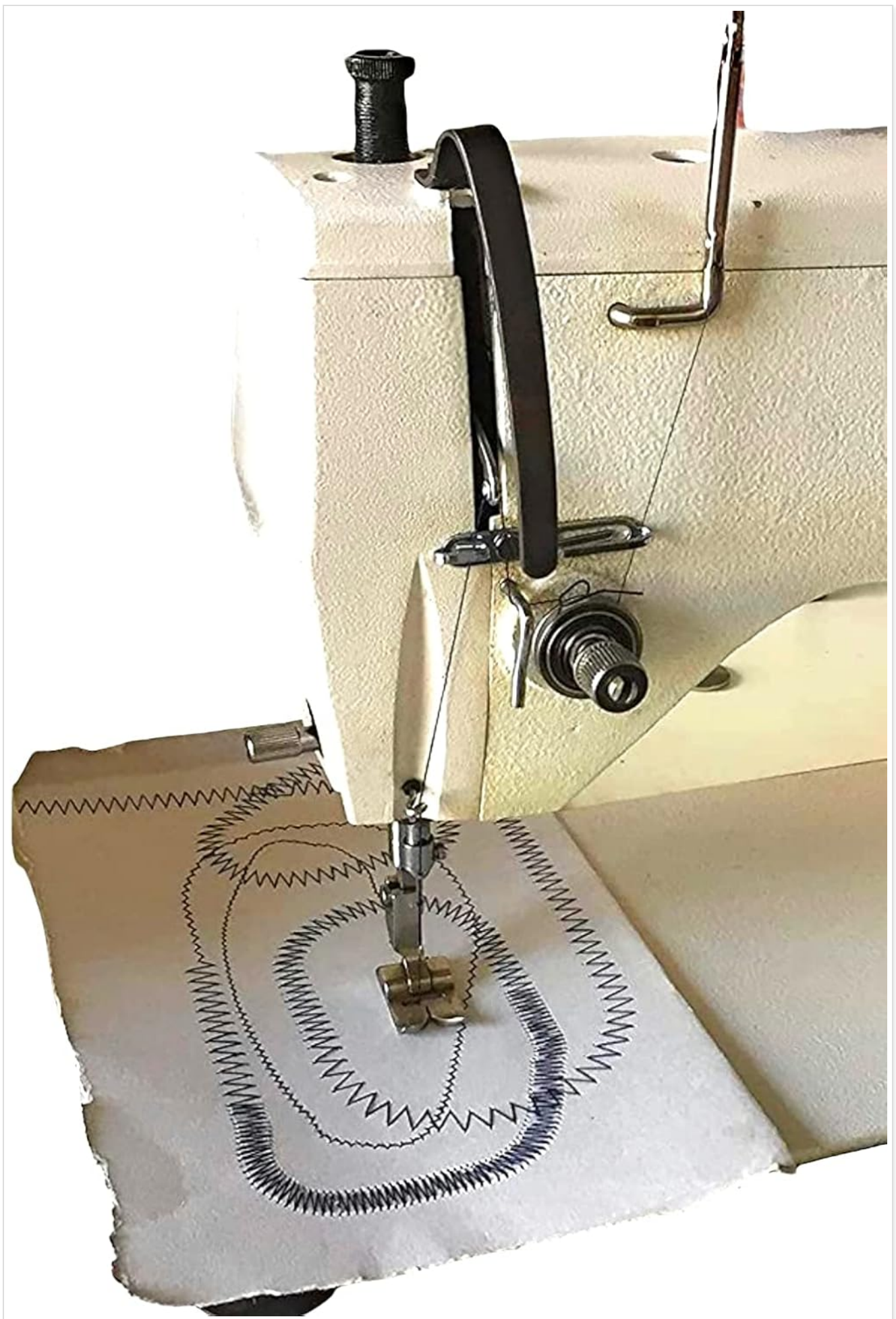
This image provides a closer look at the upper section of the sewing machine, illustrating the thread guides and tension assembly. It is useful for understanding the correct threading procedure.
