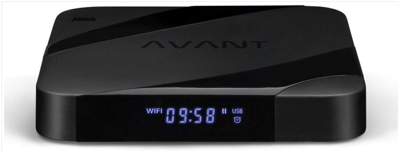
Figure 4.1: Front view of the Xsarius Avant media player, showing the digital display with time, Wi-Fi, and USB indicators.
