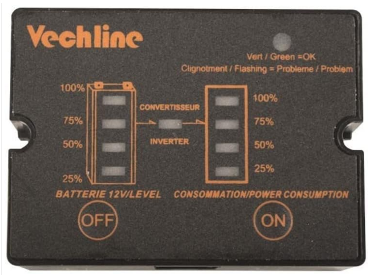
Figure 2.2: Remote Control Display. This image displays the remote control unit with indicators for battery level (12V/LEVEL) and power consumption (CONSOMMATION/POWER CONSUMPTION), along with ON/OFF buttons and status lights (Green=OK, Flashing=Problem).
