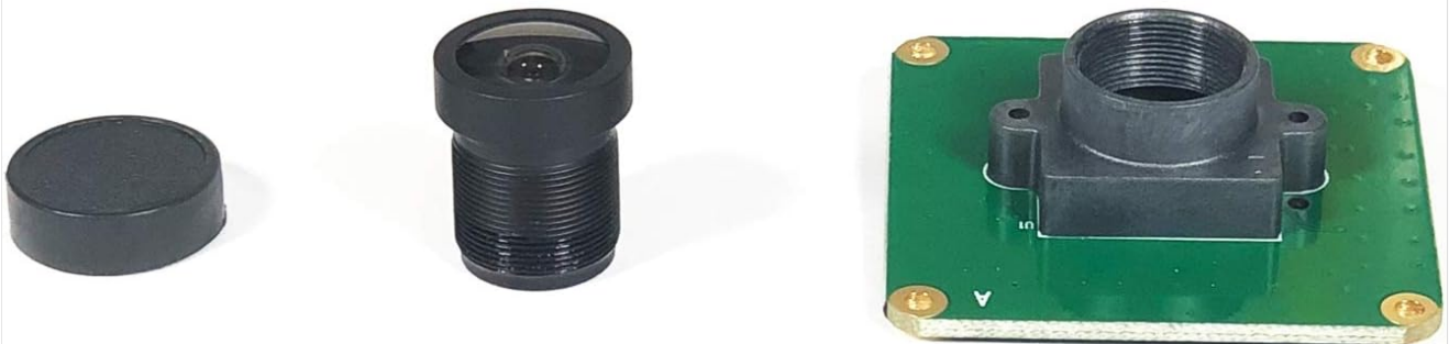
Figure 5: Demonstrates the replaceable lens feature. The lens can be unscrewed from the camera module, and the module has lens holes of 20mm with 2xD2.0mm mounting holes.
