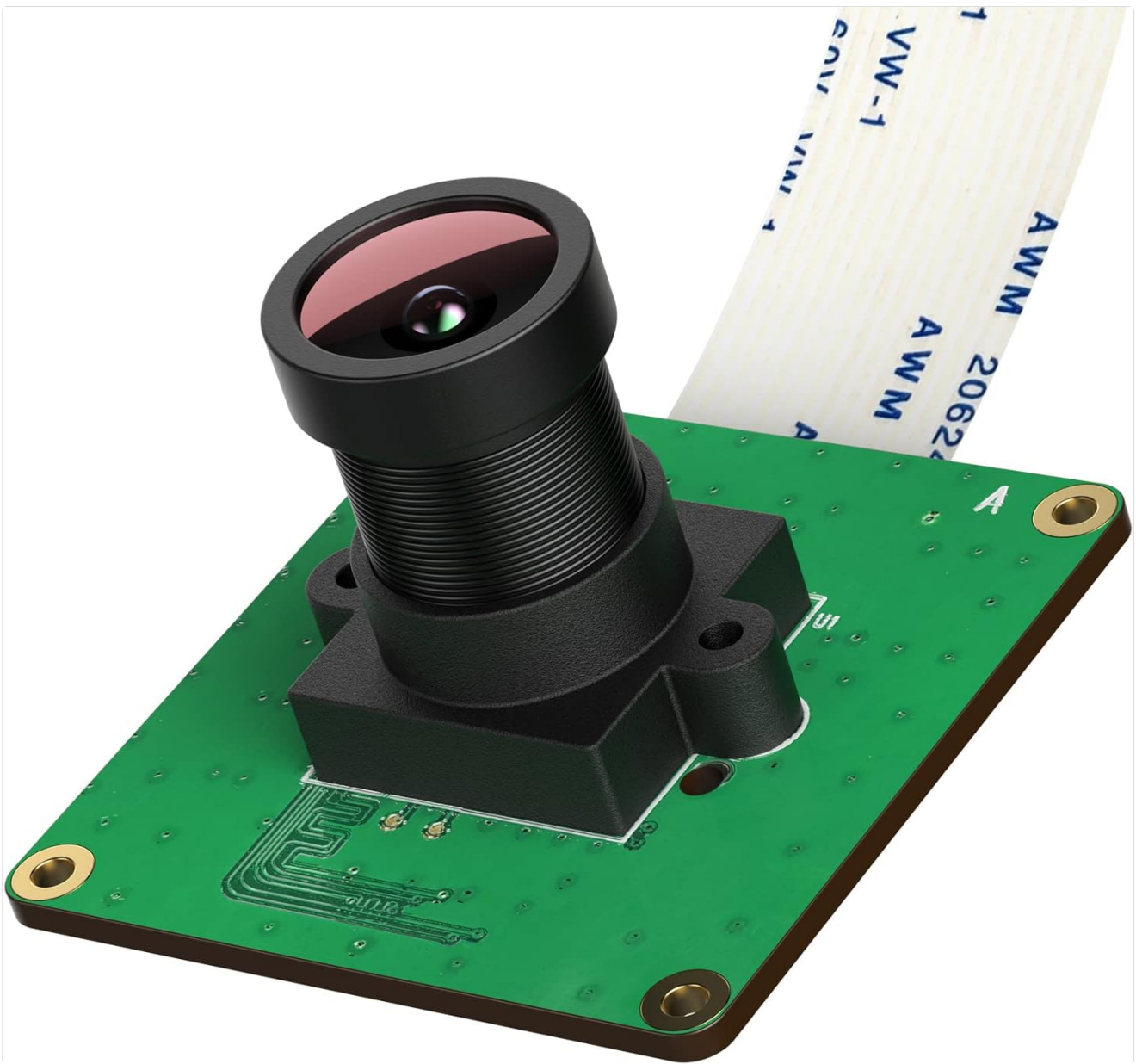
Figure 1: The innomaker CAM-MIPI327RAW Industrial Camera Module, showing the camera board with the lens assembly and the attached ribbon cable.
