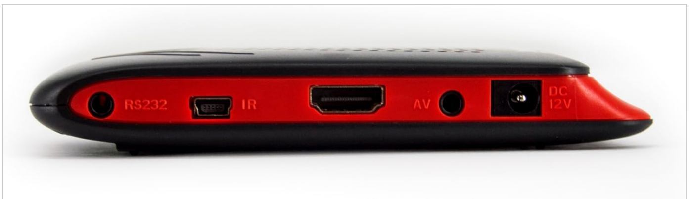
Image: The opposite side panel of the receiver, displaying the RS232 port, IR extender port, HDMI output, AV output, and DC 12V power
