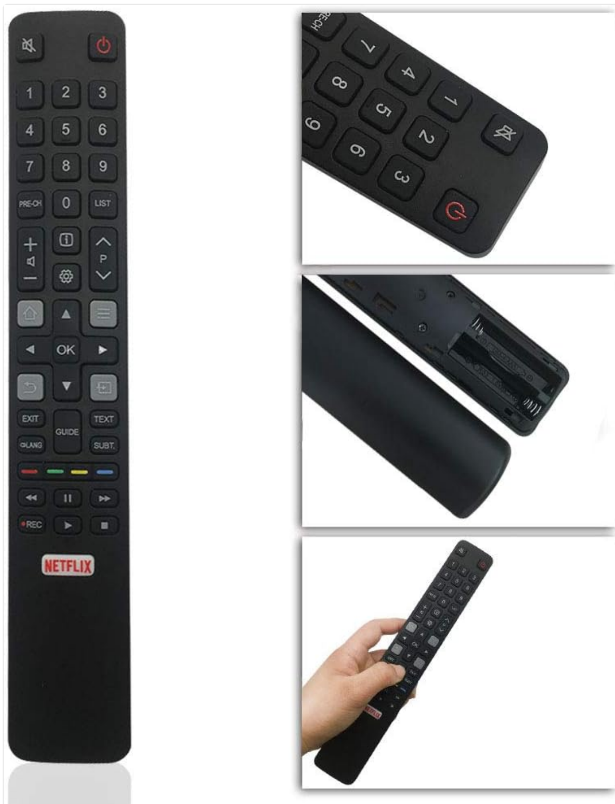
Figure 2.1: Battery compartment and installation. This image shows the back of the remote control with the battery cover removed, revealing the slots for two AAA batteries. It also shows a close-up of the remote's top section and a hand holding the remote.
