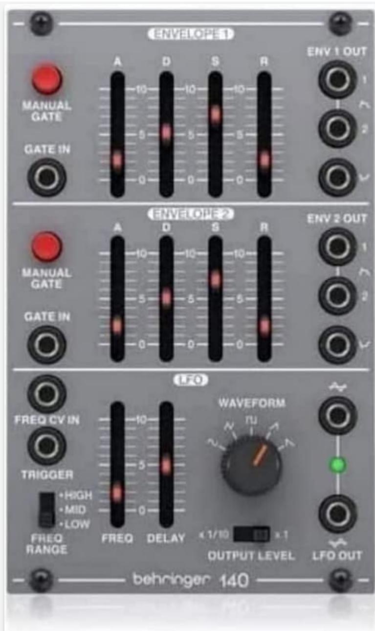
Figure 1: Front panel of the Behringer 140 Dual Envelope/LFO module. This image shows the layout of the two envelope sections at the top and middle, and the LFO section at the bottom, with all controls and jacks clearly visible.
