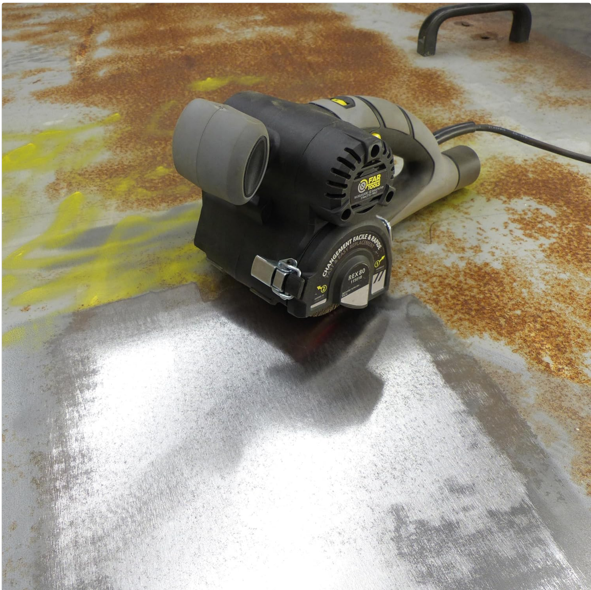
Image 4: The Fartools REX 80 in action, effectively removing rust and grime from a metal surface. This demonstrates the
