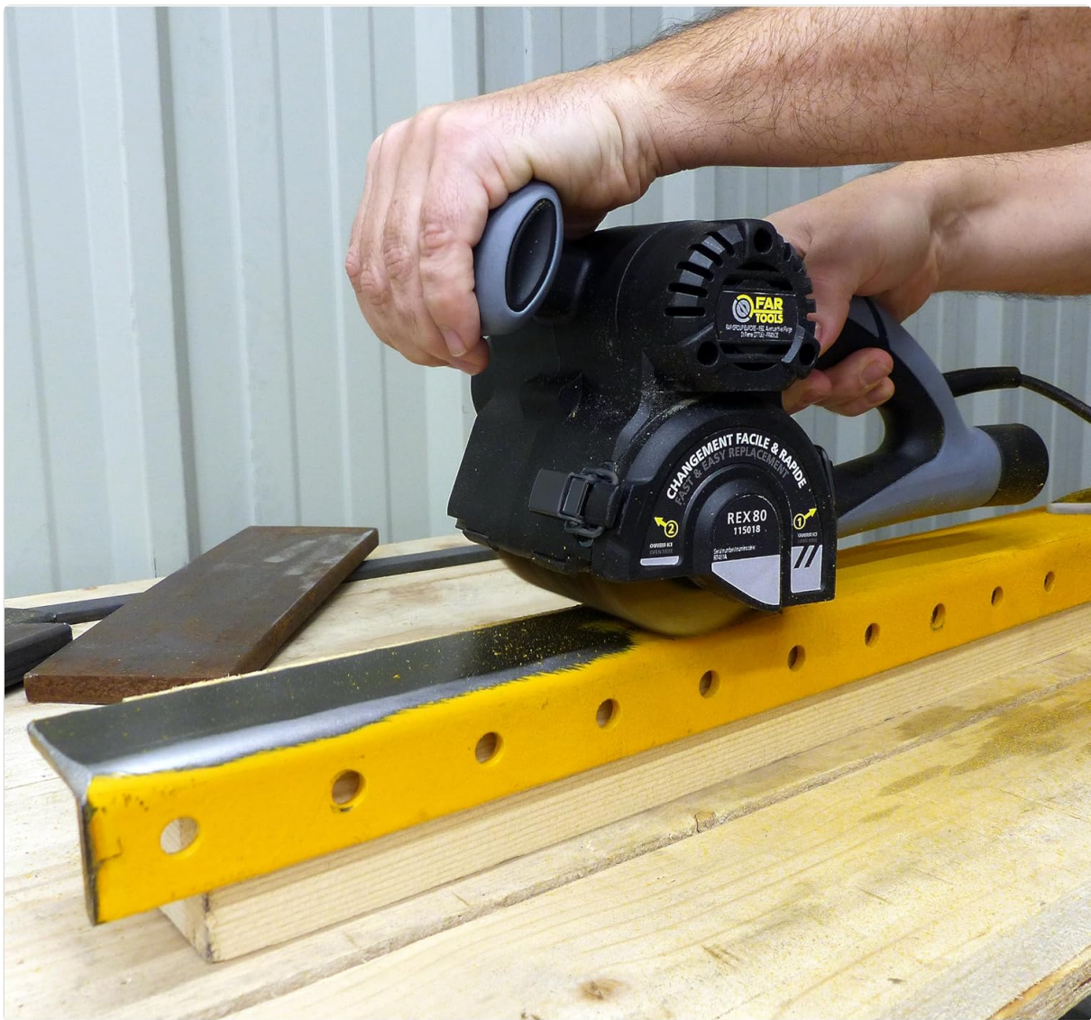
Image 6: A user operating the Fartools REX 80 with one hand on a metal beam, demonstrating the tool's lightweight and compact design allowing for single-handed use in certain applications.
