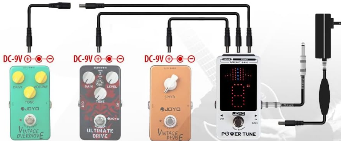
Figure 4: Connection Mode 2. This diagram shows how to connect multiple effects pedals to the JF-18R's isolated power outputs, demonstrating a typical pedalboard setup.
