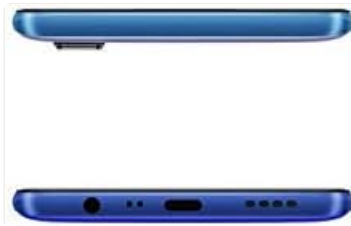
Figure 3.6: Top and bottom view of the Realme 6. The bottom edge includes the 3.5mm headphone jack, USB Type-C port, microphone, and speaker grille.
