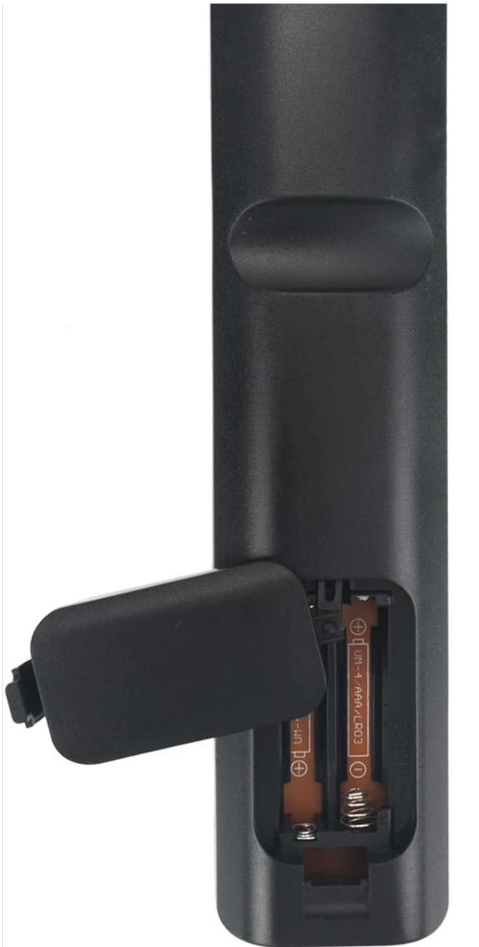
Figure 1: Rear view of the remote control with the battery compartment open for AAA battery insertion. The remote control is now ready for use. No additional programming or pairing is required.
