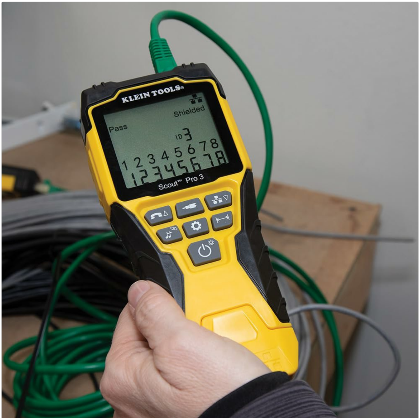
Figure 4: Testing an Ethernet cable with the Scout Pro 3 Tester.
