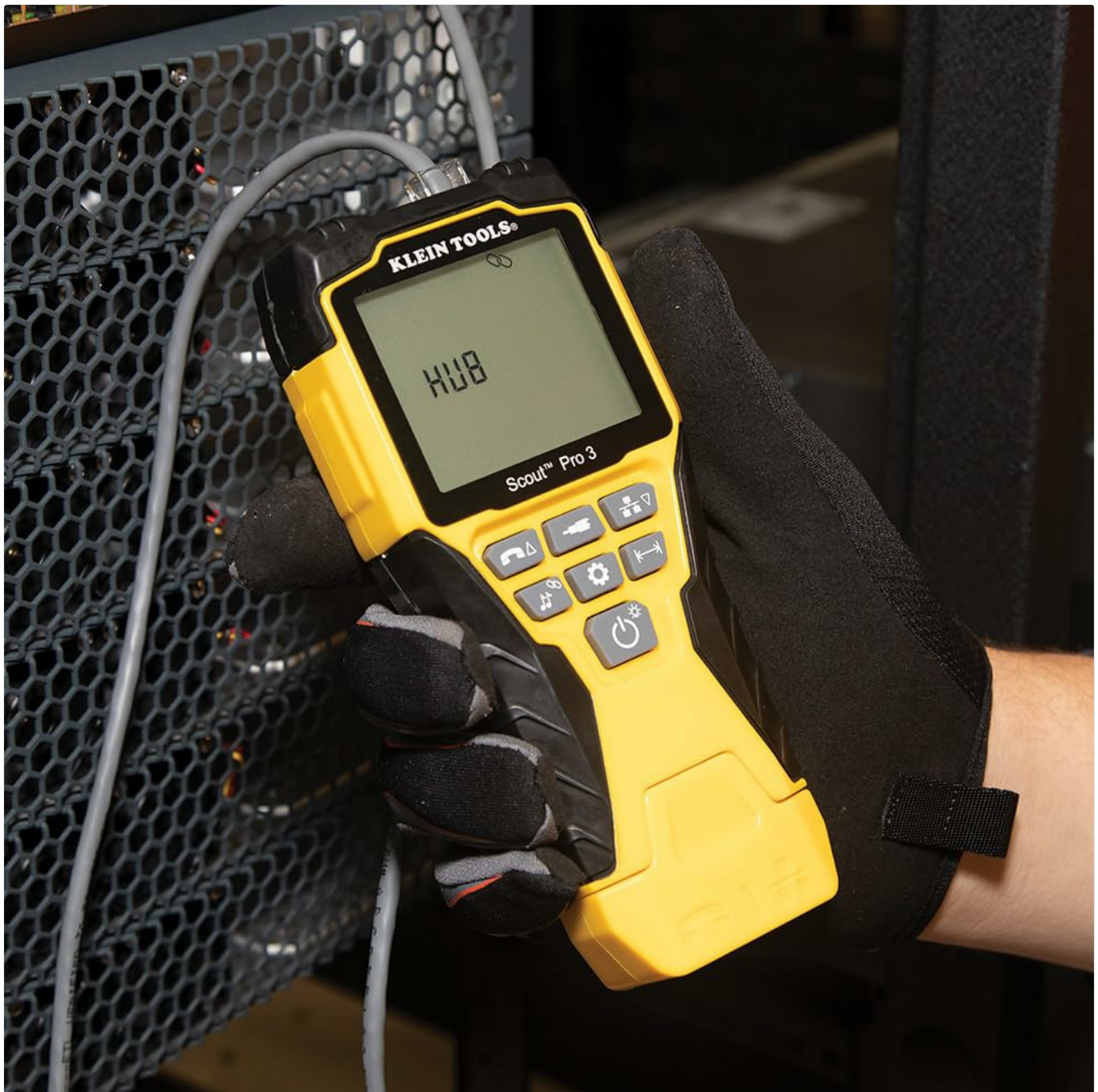
Figure 8: Using Hub Blink mode to identify a port on a network switch.
