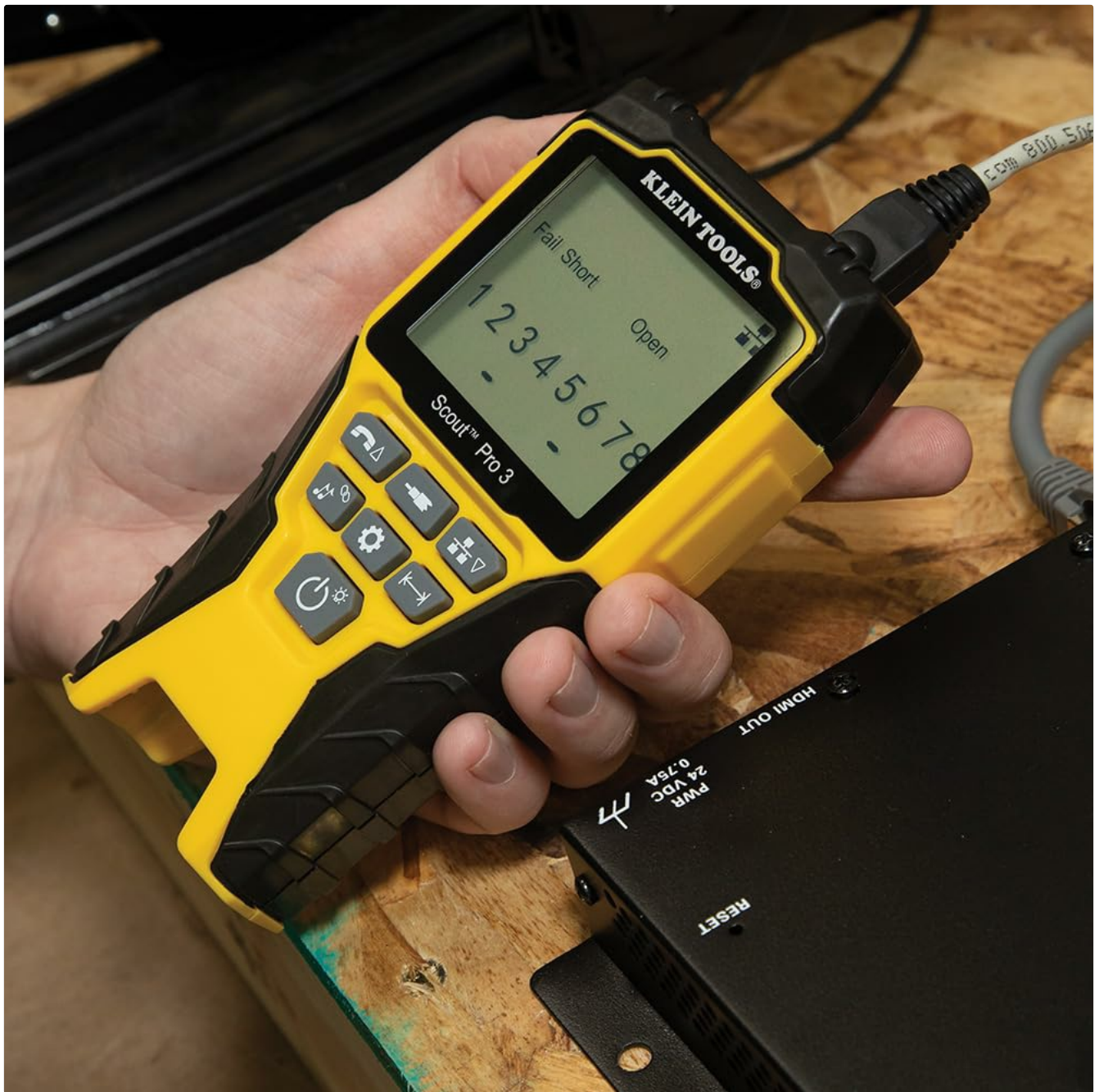
Figure 9: The display indicates specific cable faults like "Fail Short" for easy diagnosis.
