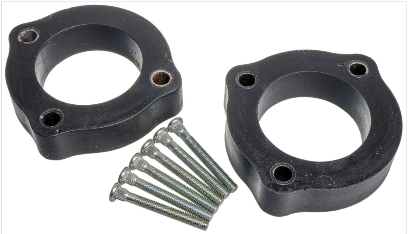
Figure 3.2: Rear strut spacers and associated bolts, used to lift the rear suspension.
