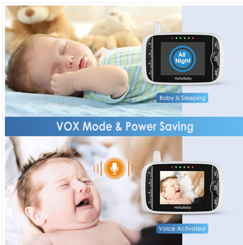
Image: VOX mode activates the monitor screen only when sound is detected, saving power.
