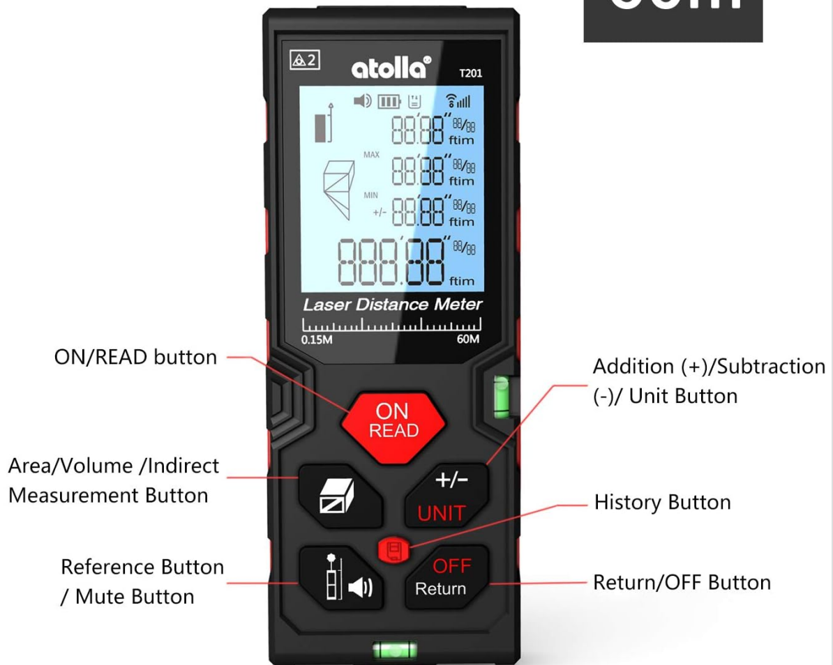
Figure 2: Front view of the atolla T201 with labeled buttons.
