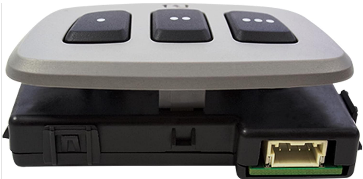
Image 2: Side view of the Advent Homelink 5 unit, illustrating the electrical connector for vehicle integration.
