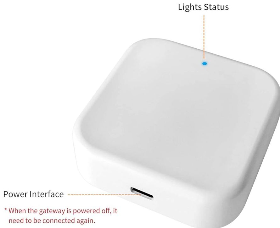
Image: Diagram showing the G2 Gateway's power interface and the meaning of its blue and red indicator lights.
