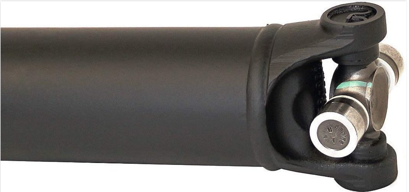
Figure 2: Close-up view of a driveshaft universal joint, highlighting the new components.
