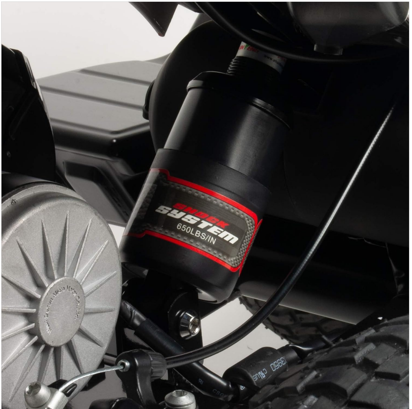
Figure 6.1: Suspension system. This image shows a close-up of the quad's suspension, which should be checked for proper function and wear.
