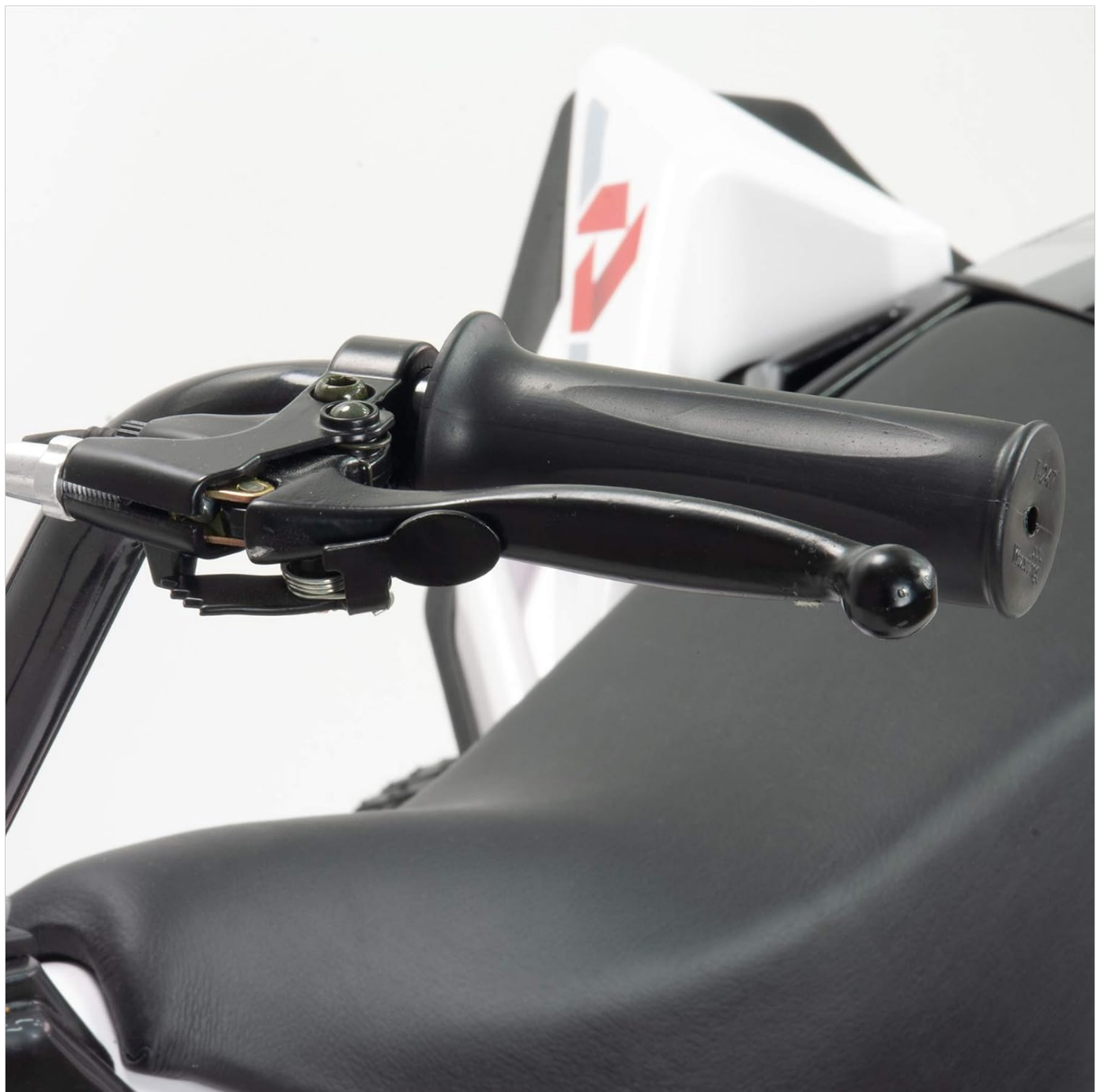
Figure 5.3: Close-up of the brake lever. This image details the brake lever mechanism on the left handlebar.
