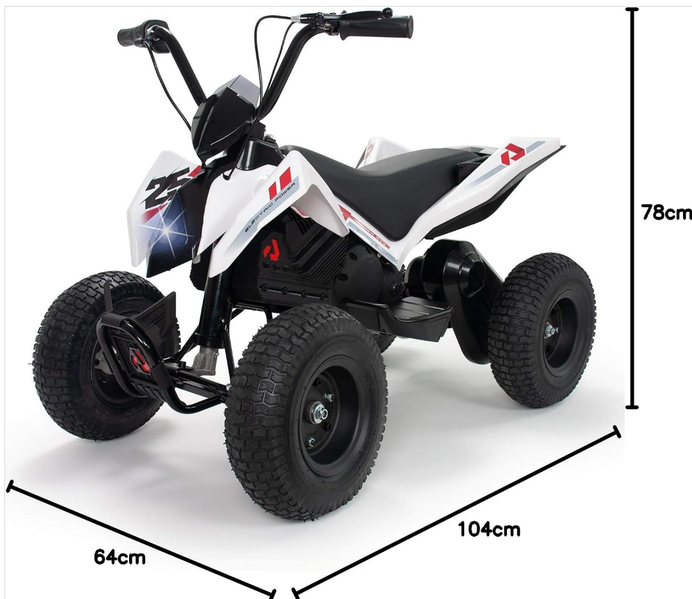
Figure 8.1: Dimensions of the INJUSA X-Treme Zero 24V Electric Quad. This image illustrates the length, width, and height of the quad.
