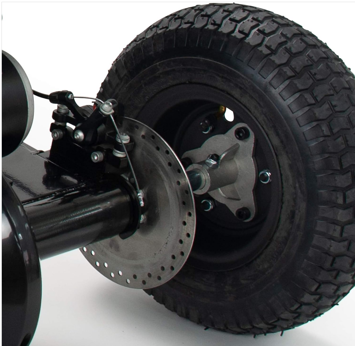
Figure 5.4: Rear disc brake and wheel. This image provides a detailed view of the disc brake system on the rear wheel.
