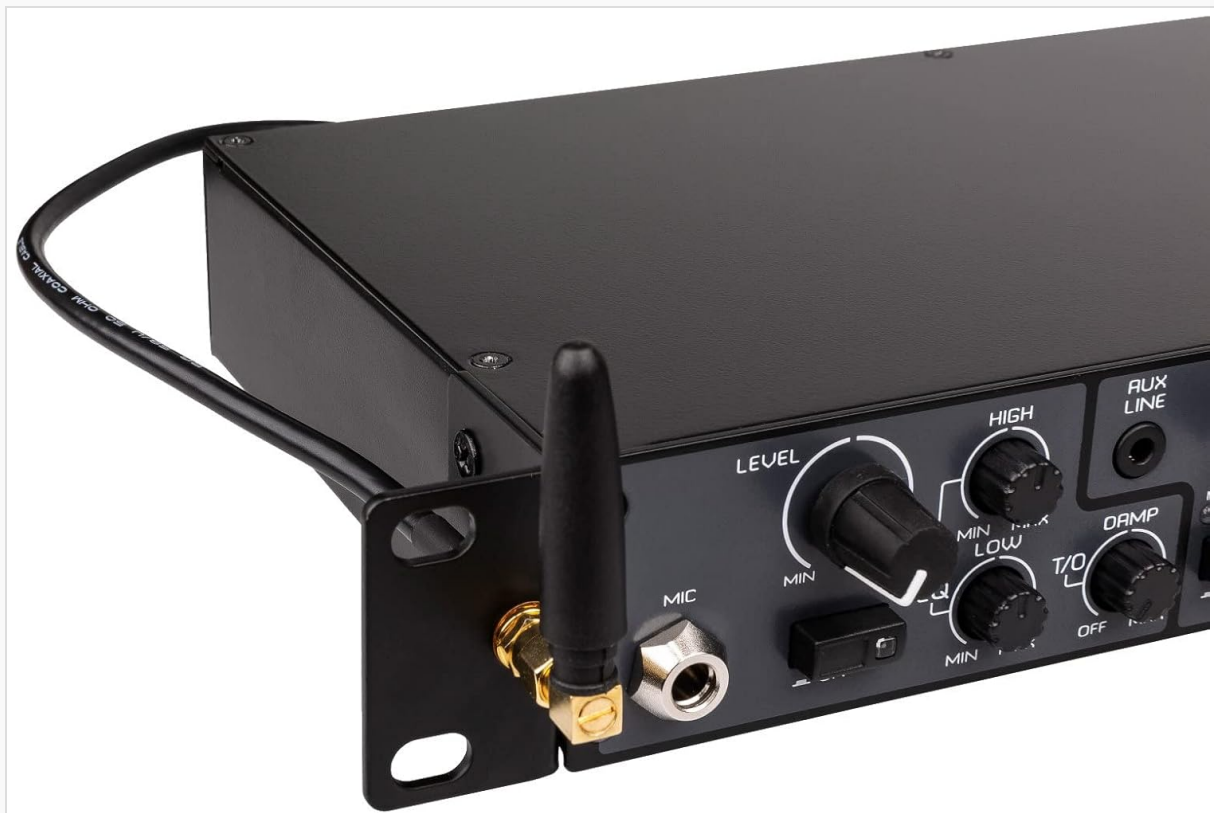
Figure 4.2: Left side of the front panel. This close-up highlights the microphone input, its level control, and the high/low EQ knobs.
