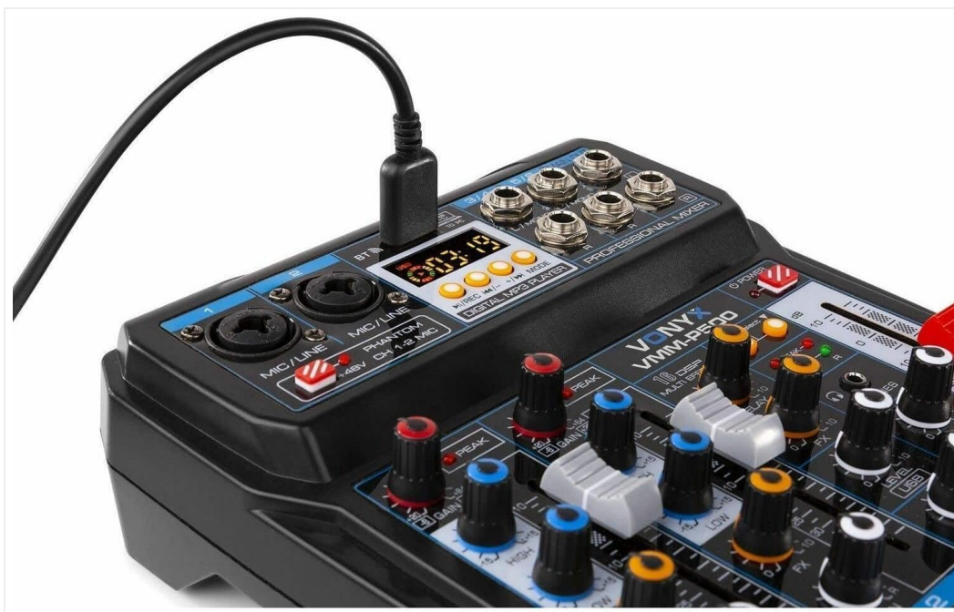
Figure 4: USB-A cable connected to the "TO PC" port on the VMM-P500 mixer, enabling connection to a computer for audio interface functionality.
