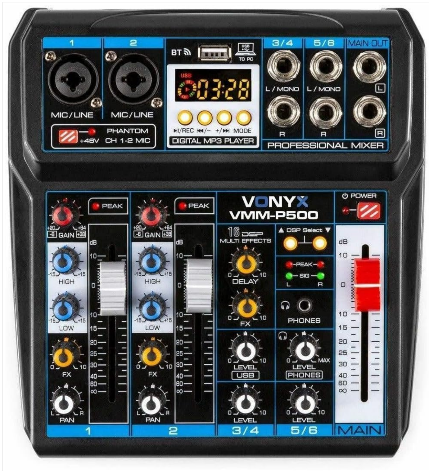
Figure 1: Top view of the Vonyx VMM-P500 mixer, highlighting the microphone/line inputs, USB/MP3 player section, main output, and various channel controls including gain, EQ, effects, and pan, along with the main fader.
