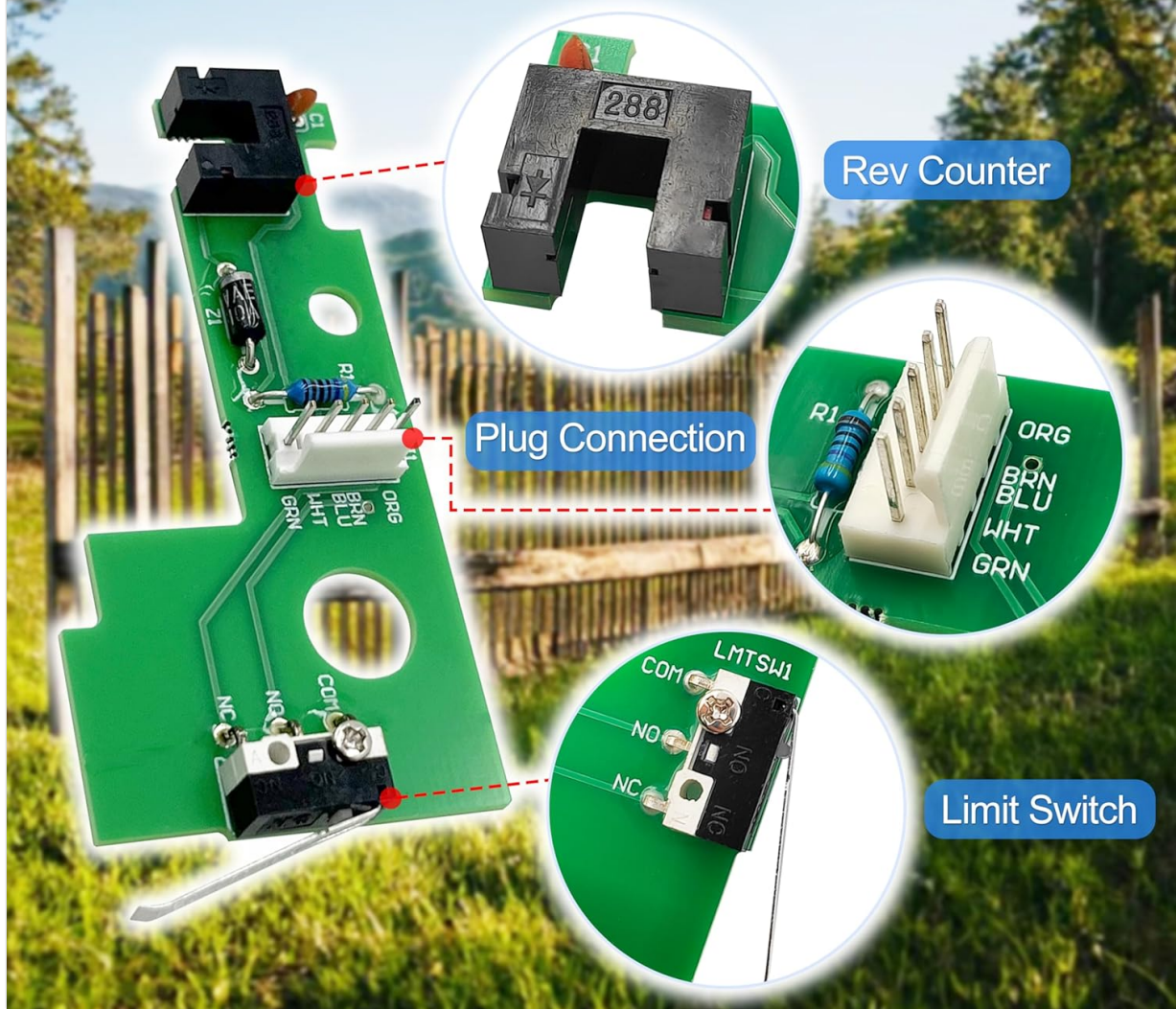
Image 1.2: Close-up view highlighting the Rev Counter sensor, the plug connection, and the limit switch on the board.
