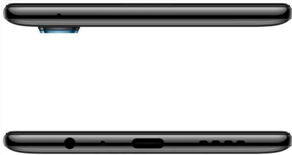
Figure 2.2: Bottom view of the realme 6 Pro, illustrating the USB Type-C charging port and 3.5mm headphone jack.
