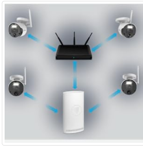
Image: A diagram illustrating multiple wireless cameras connecting to a central NVR unit via a router, demonstrating the wireless setup.
