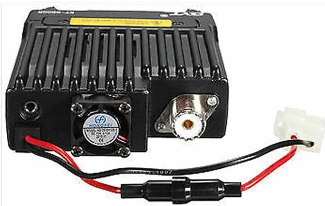
Figure 3.5: Rear view of the KT-8900R, showing the cooling fan, antenna connector, and power input.
