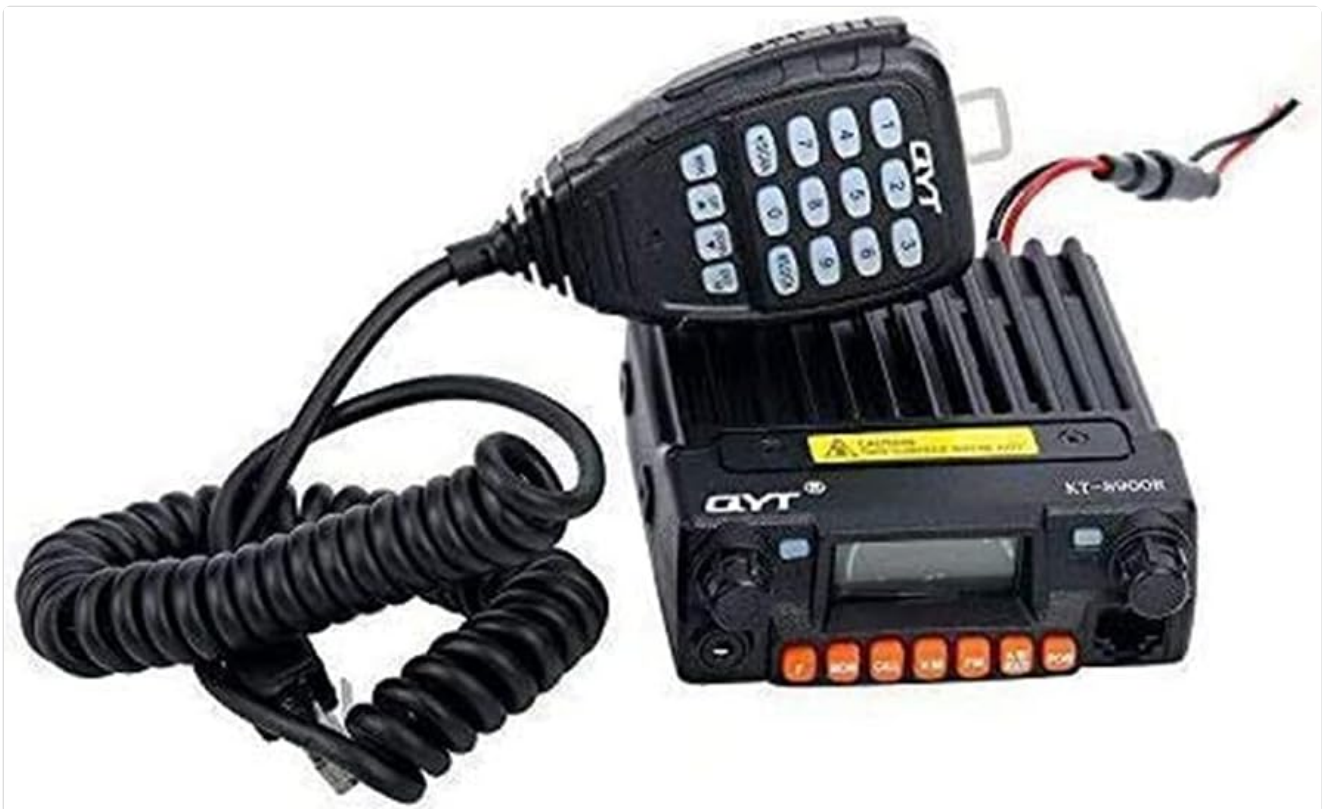
Figure 4.1: The KT-8900R radio unit with the microphone properly connected to the front panel.
