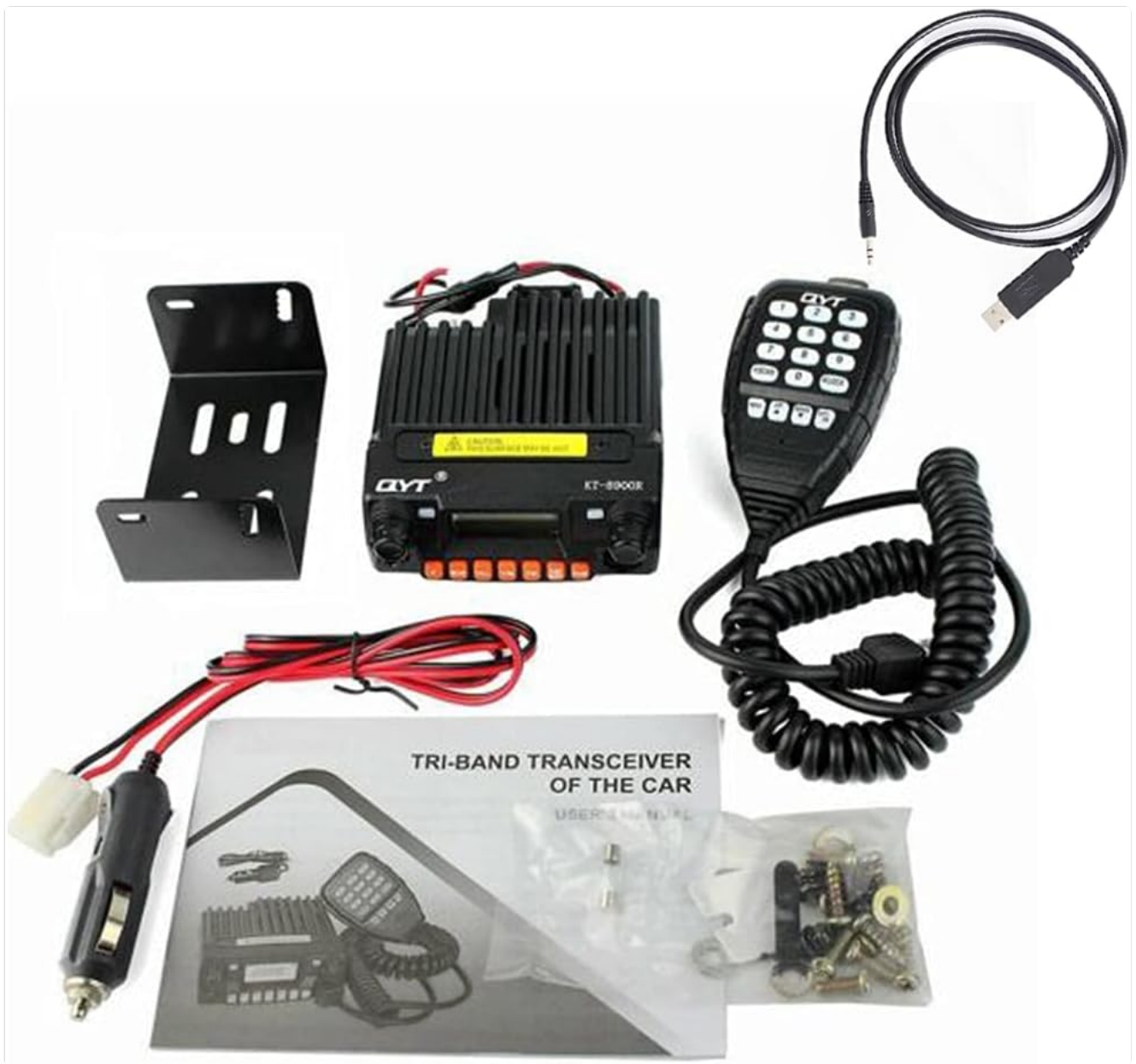
Figure 2.1: All components included in the QYT KT-8900R package, including the radio unit, microphone, power cable, mounting bracket, and programming cable.
