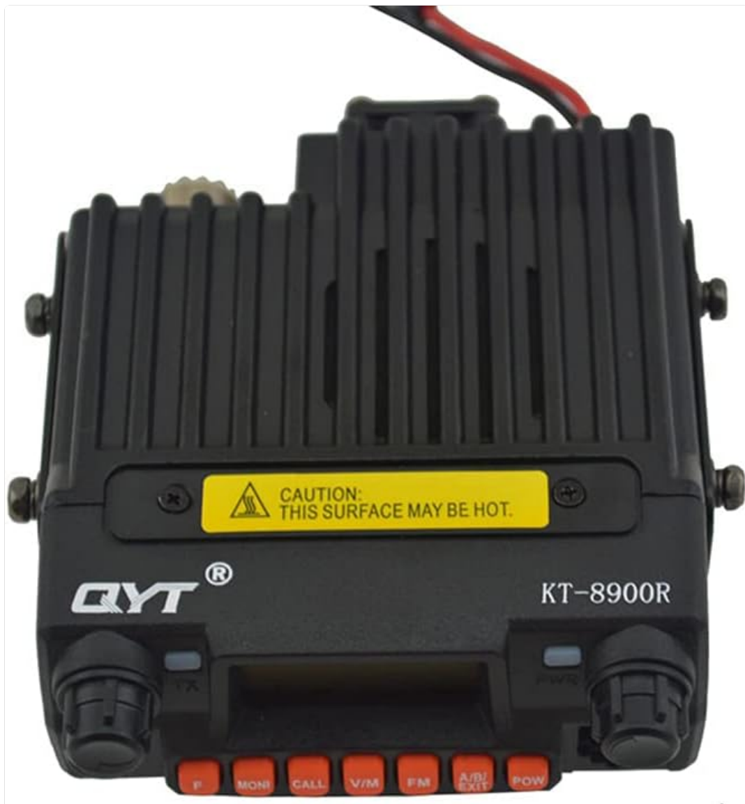
Figure 3.1: Front view of the KT-8900R radio unit, showing the display, control knobs, and function buttons.
