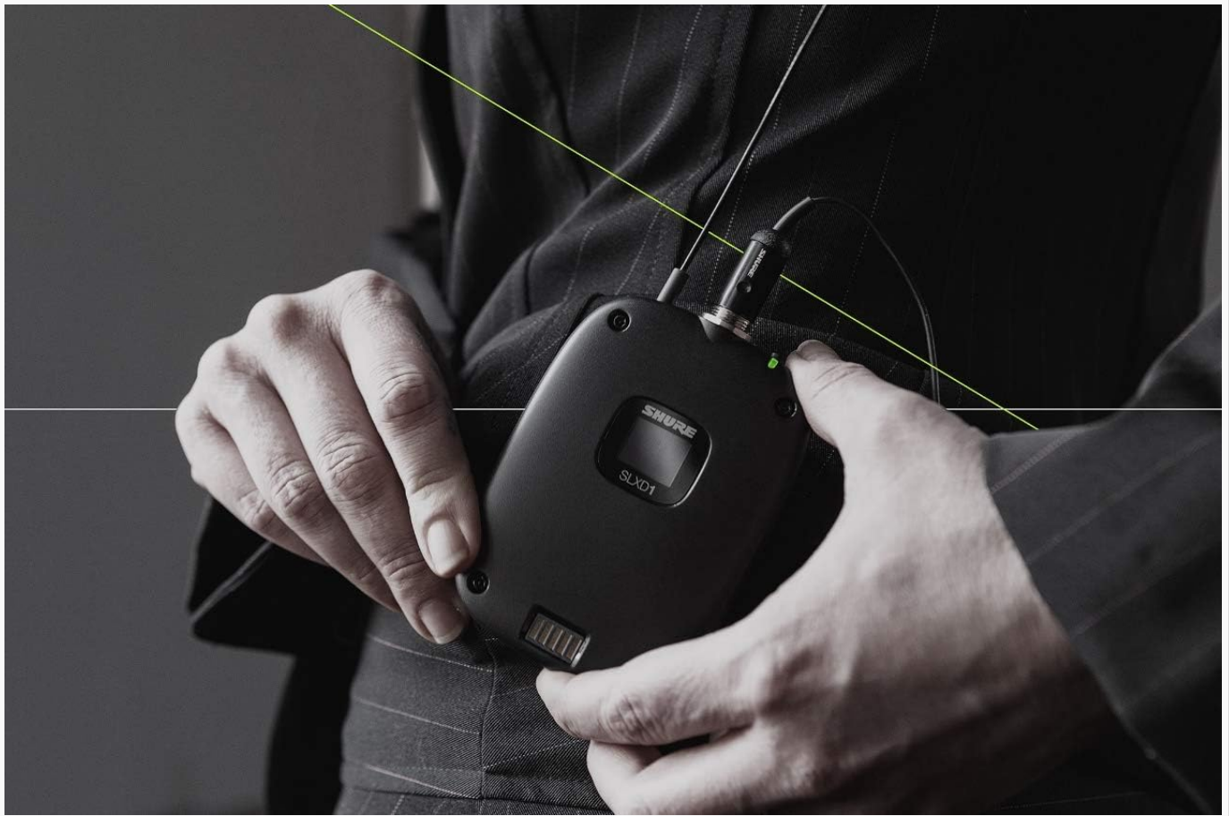
Figure 3: A person wearing the SLXD1 Bodypack Transmitter clipped to their clothing, demonstrating typical placement during use.
