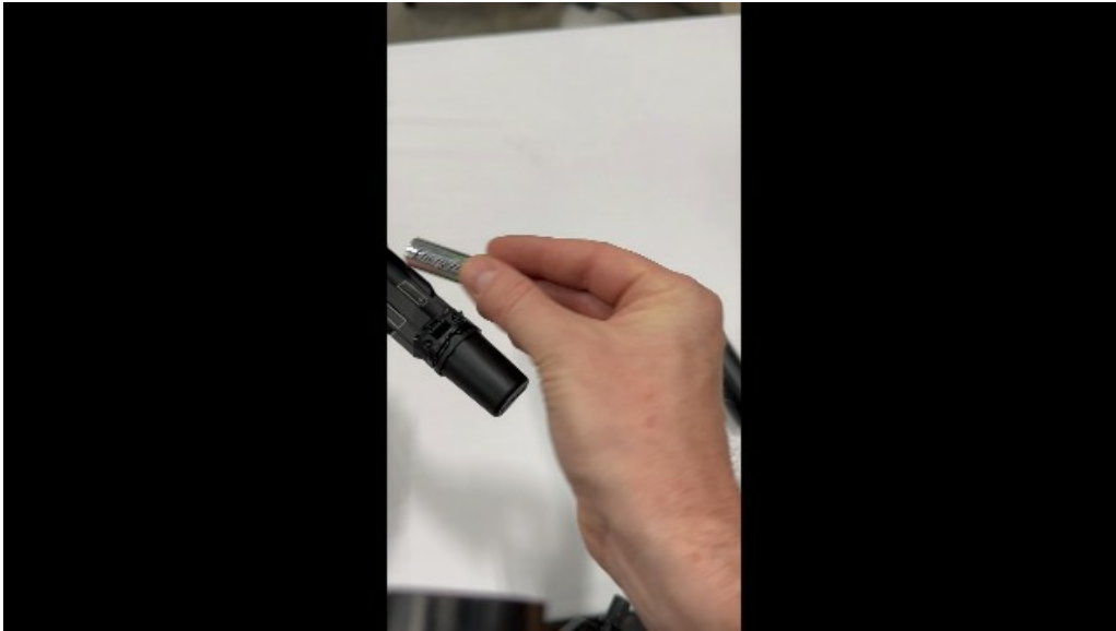
Figure 2: Battery installation in the SLXD2/SM58 transmitter.
