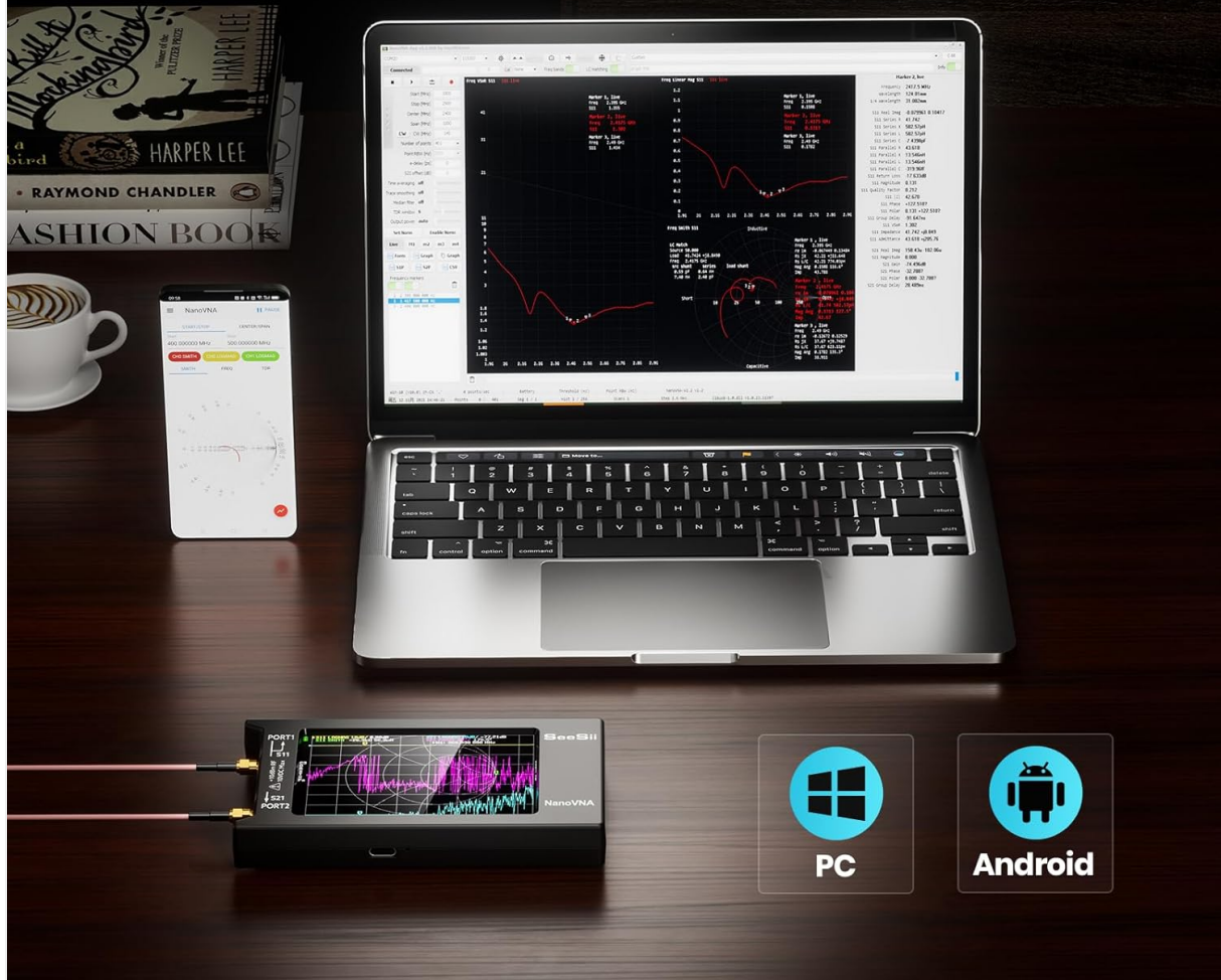
Figure 4: NanoVNA-H4 connected to a PC and an Android phone for advanced control and data visualization.
