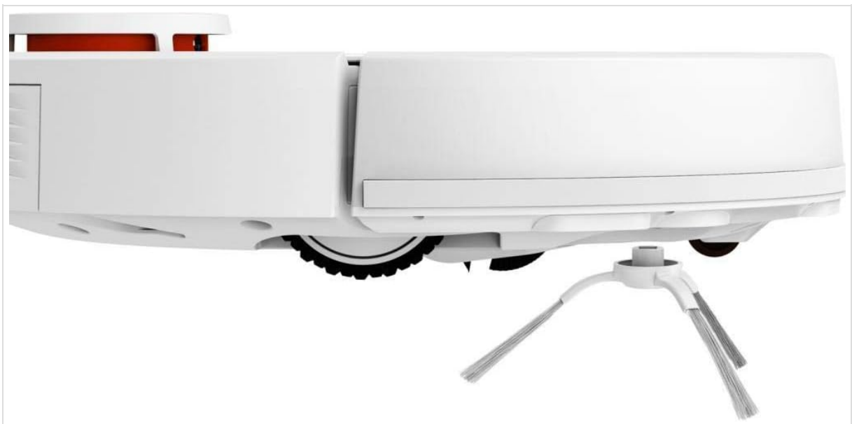
Image Description: Side profile of the Xiaomi Mijia Robot Vacuum Cleaner, highlighting one of the side brushes and a main wheel.
