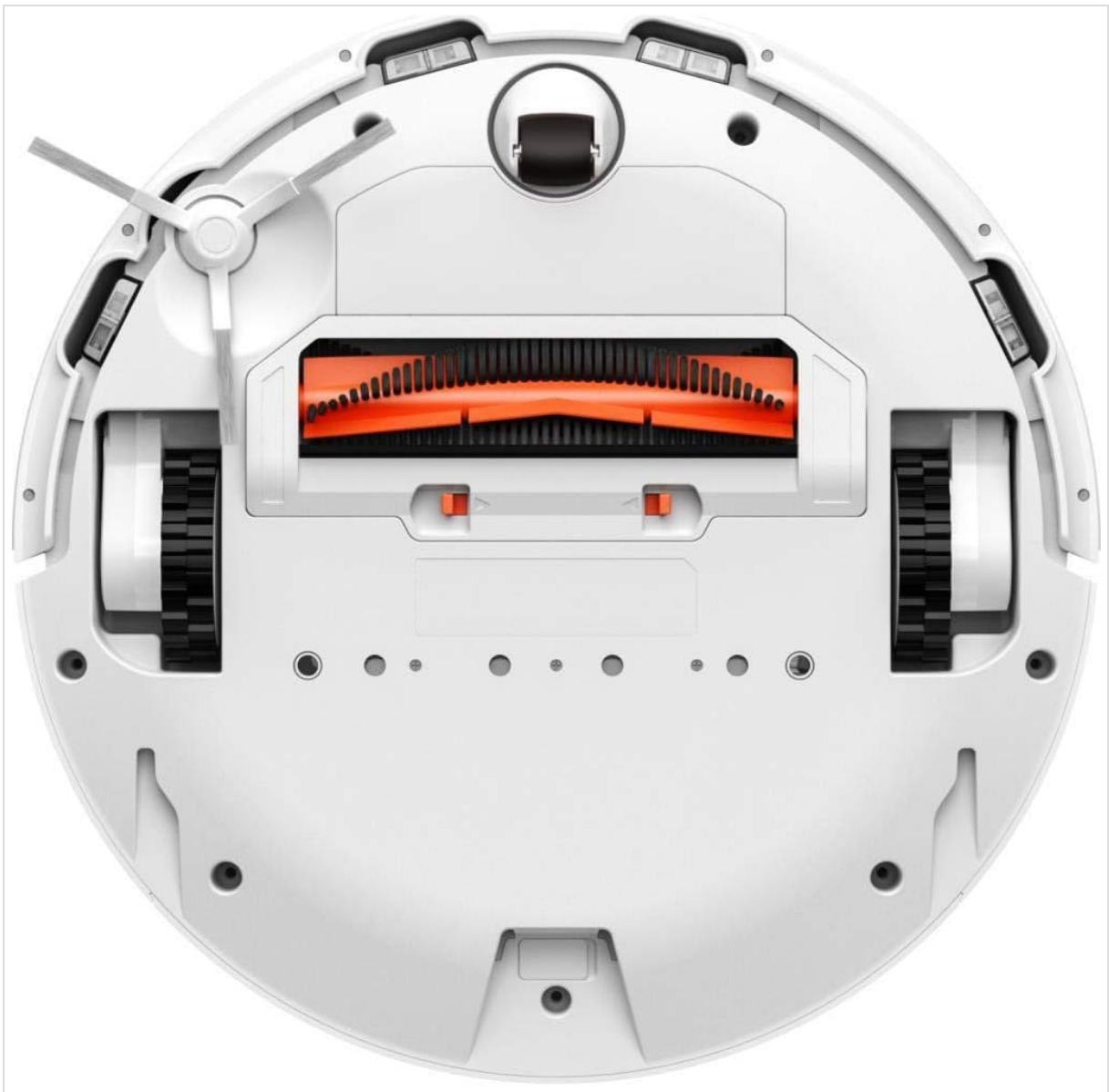
Image Description: Bottom view of the Xiaomi Mijia Robot Vacuum Cleaner, displaying the main roller brush (orange), side brushes, charging contacts, and various sensors.
