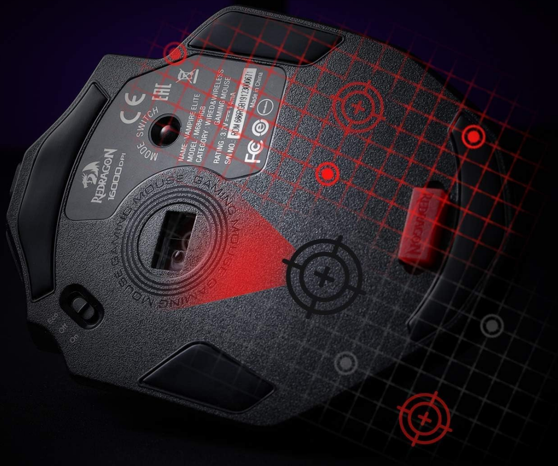
Image 8.1: The underside of the Redragon M686 mouse, highlighting the PAW3335 optical sensor.
