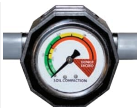
Figure 2: Detailed view of the water-filled stainless steel dial, featuring color-coded zones (Green, Yellow, Red) to indicate compaction levels.
