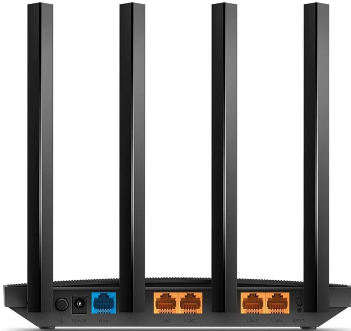
Figure 1.2: Rear view of the Archer C80 router. From left to right, it shows the power button, power input, a blue Gigabit WAN port, four yellow Gigabit LAN ports, and a WPS/Wi-Fi button, and a reset button.
