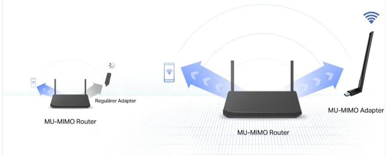
Figure 5.1: Illustration of MU-MIMO technology, demonstrating simultaneous data streams to multiple devices.
