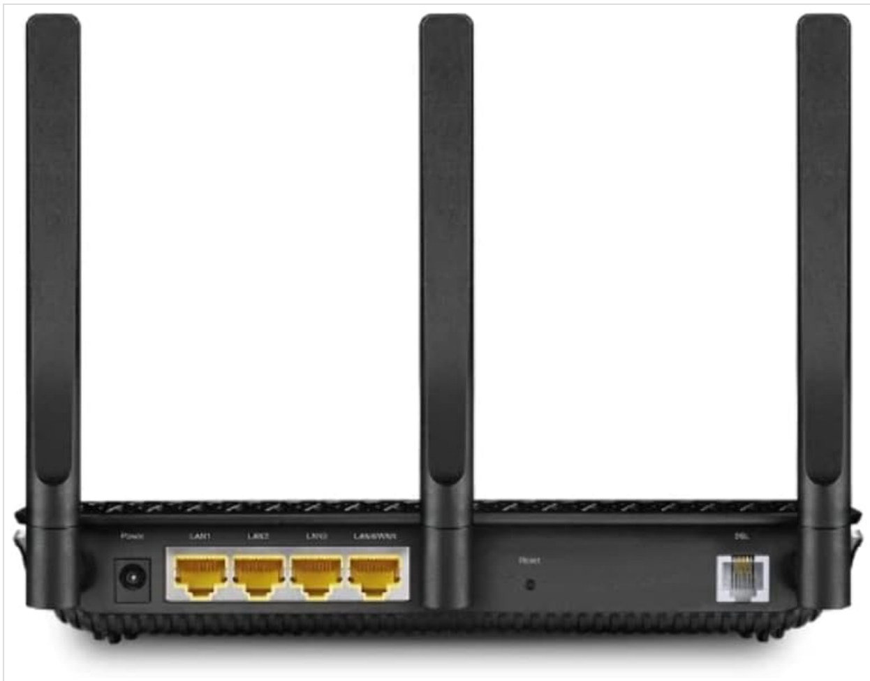
Image: Rear view of the Archer VR2100, displaying the power input, four Gigabit LAN ports, one LAN/WAN port, a Reset button, a USB 3.0 port, and a DSL port.
