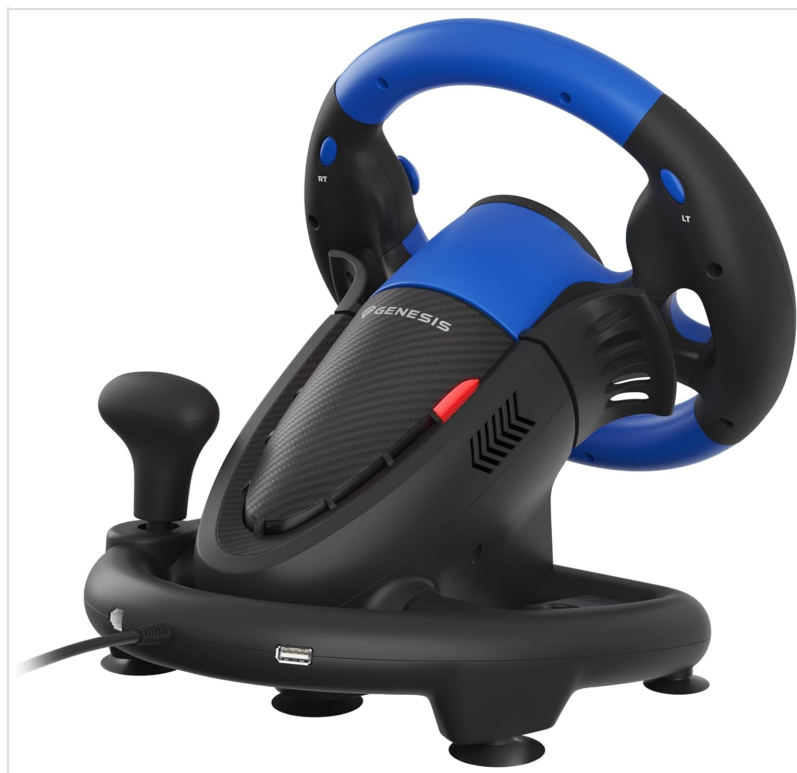
Figure 3.1: The rear view of the racing wheel unit, illustrating the integrated USB cable for connection to gaming platforms and the port for the pedal unit.
