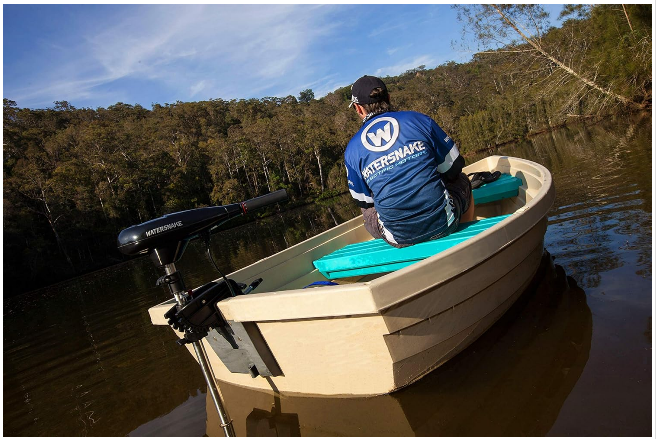
Figure 3: The Watersnake Tracer Trolling Motor securely mounted on the transom of a small boat.
