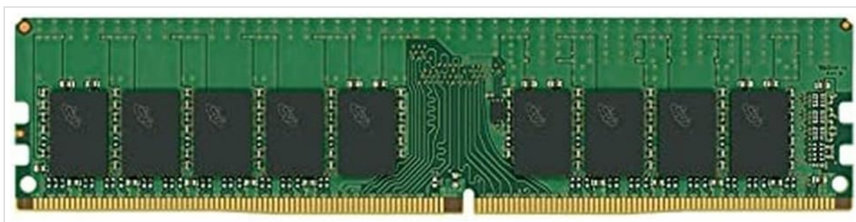
Image: Crucial Micron 32GB DDR4 SDRAM Memory Module. This image displays the green circuit board with black memory chips and gold contacts along the bottom edge, ready for insertion into a DIMM slot.
