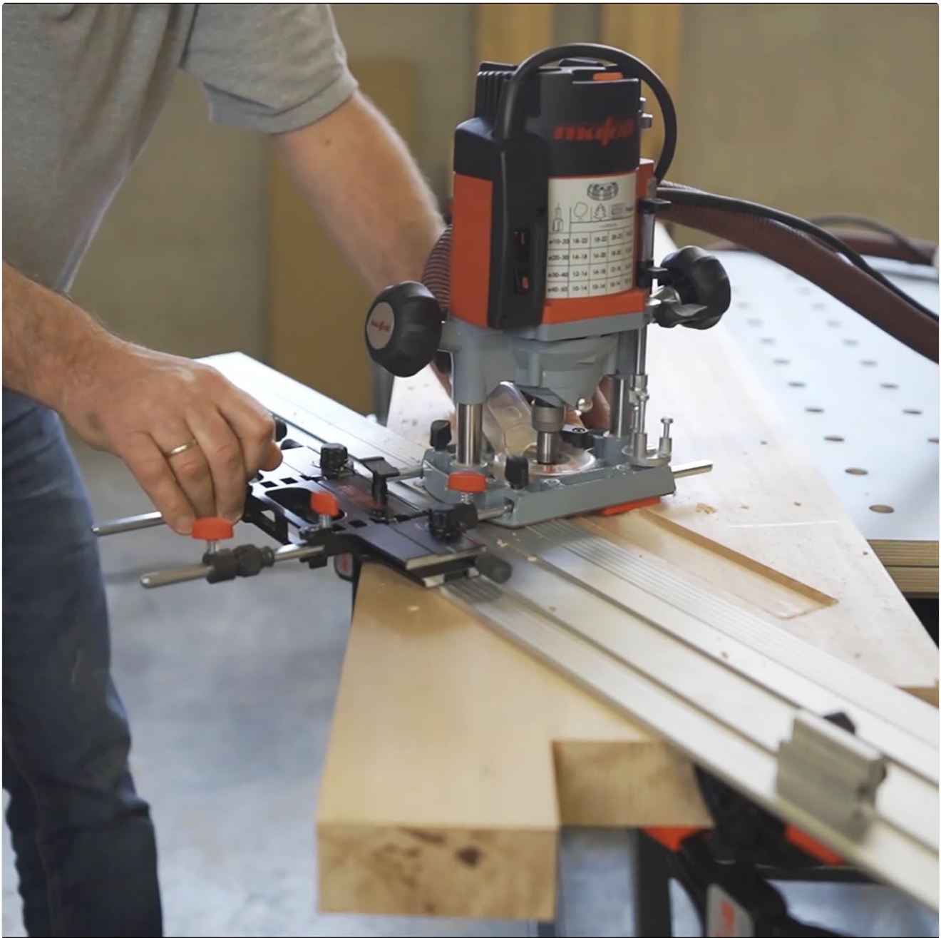
Figure 5.2: The Mafell LO-FA 207200 Router Adapter being used to guide the router along a straight edge of a workpiece. The adjustable stop jaws maintain a consistent distance from the edge.
