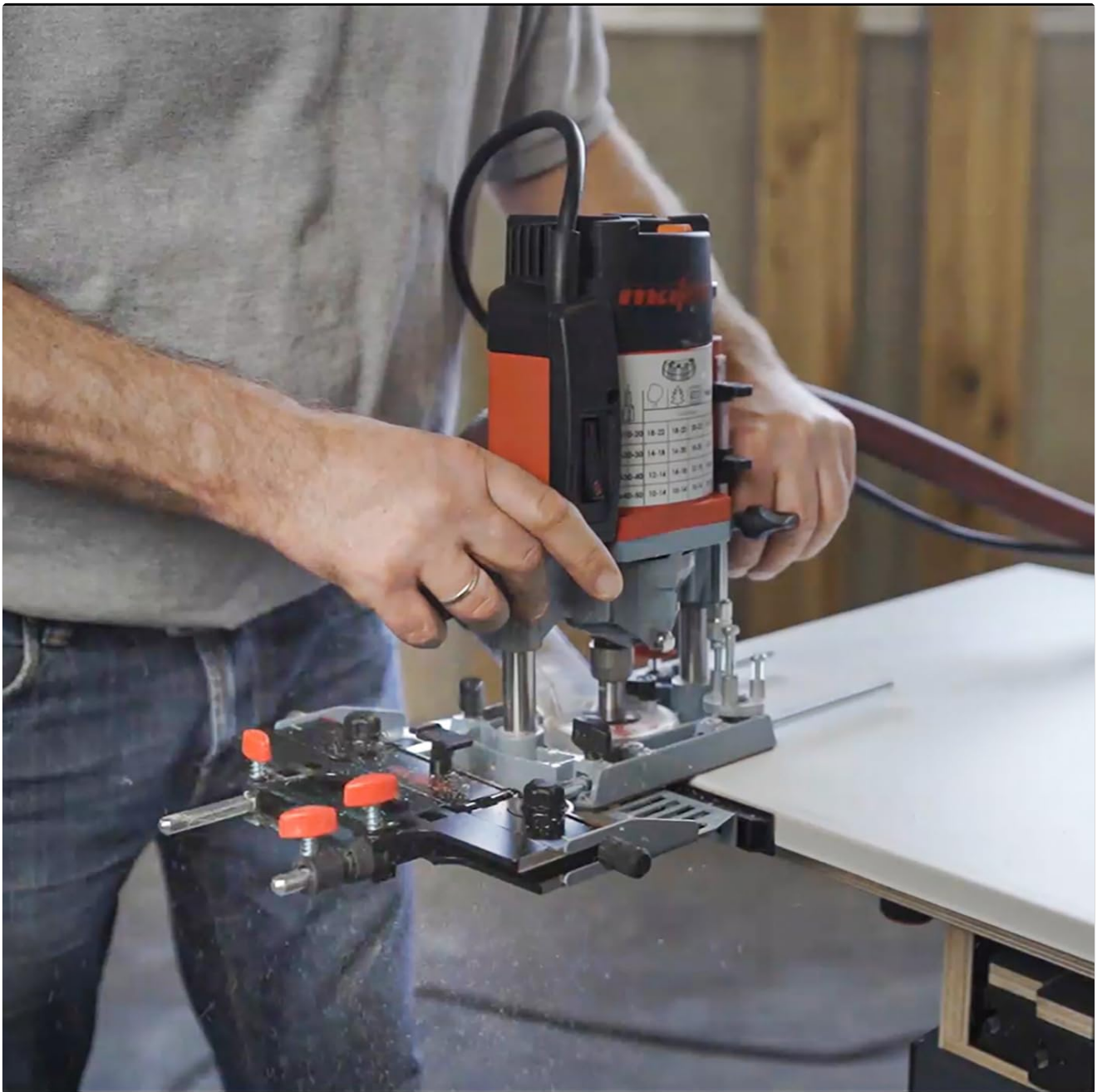
Figure 5.3: A closer view of the Mafell LO-FA 207200 Router Adapter during operation, highlighting the router's position relative to the adapter and the importance of dust management.
