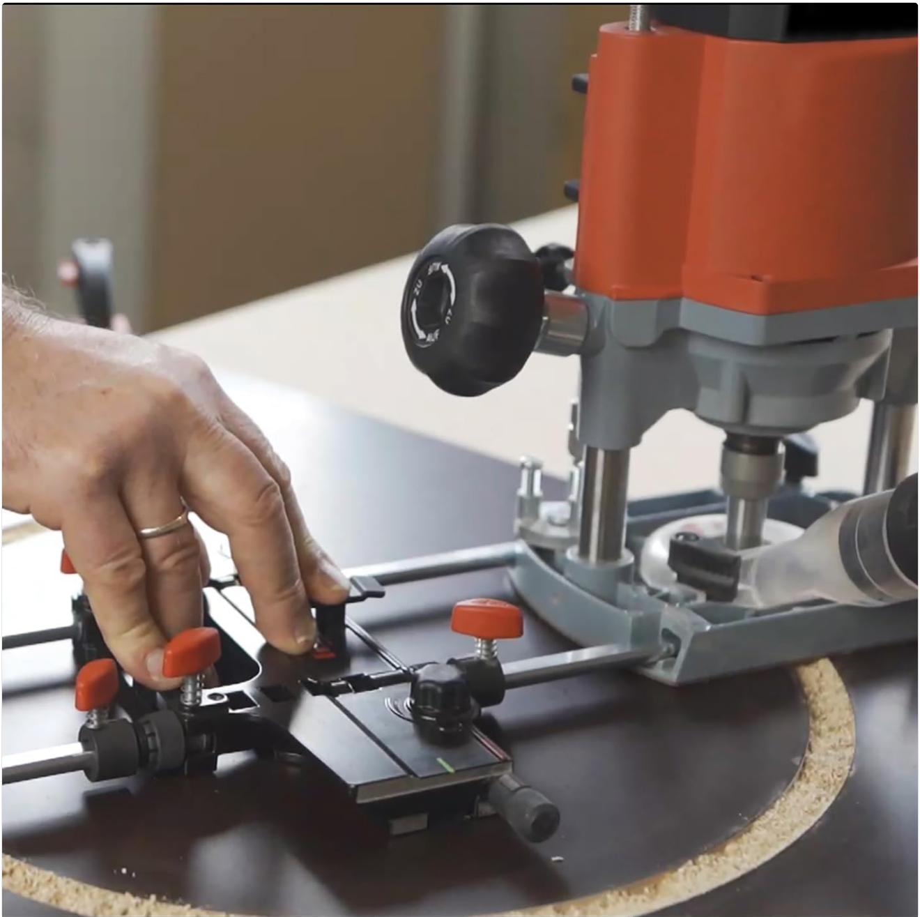
Figure 5.1: The Mafell LO-FA 207200 Router Adapter in use for cutting a precise circle. The compass pin acts as a pivot point, guiding the router along the desired radius.
