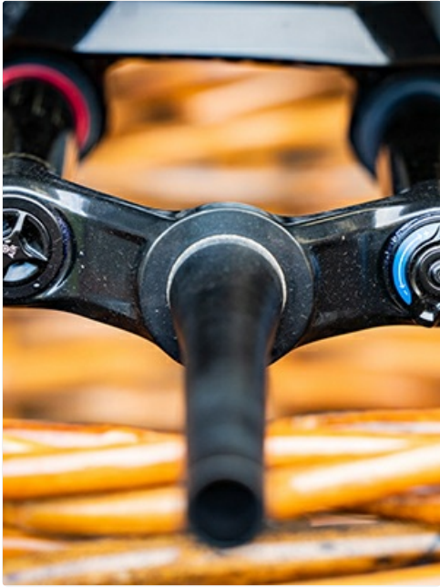
Close-up view of the fork crown, showing the air valve cap and lockout lever for adjustments.
