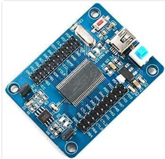
Figure 2: Close-up of the development board, highlighting the CY7C68013A-56 chip and pin headers.
