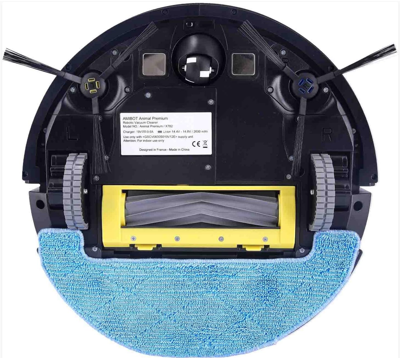
Image: Bottom view of the robot, displaying the main brush, side brushes, wheels, and mop attachment.
