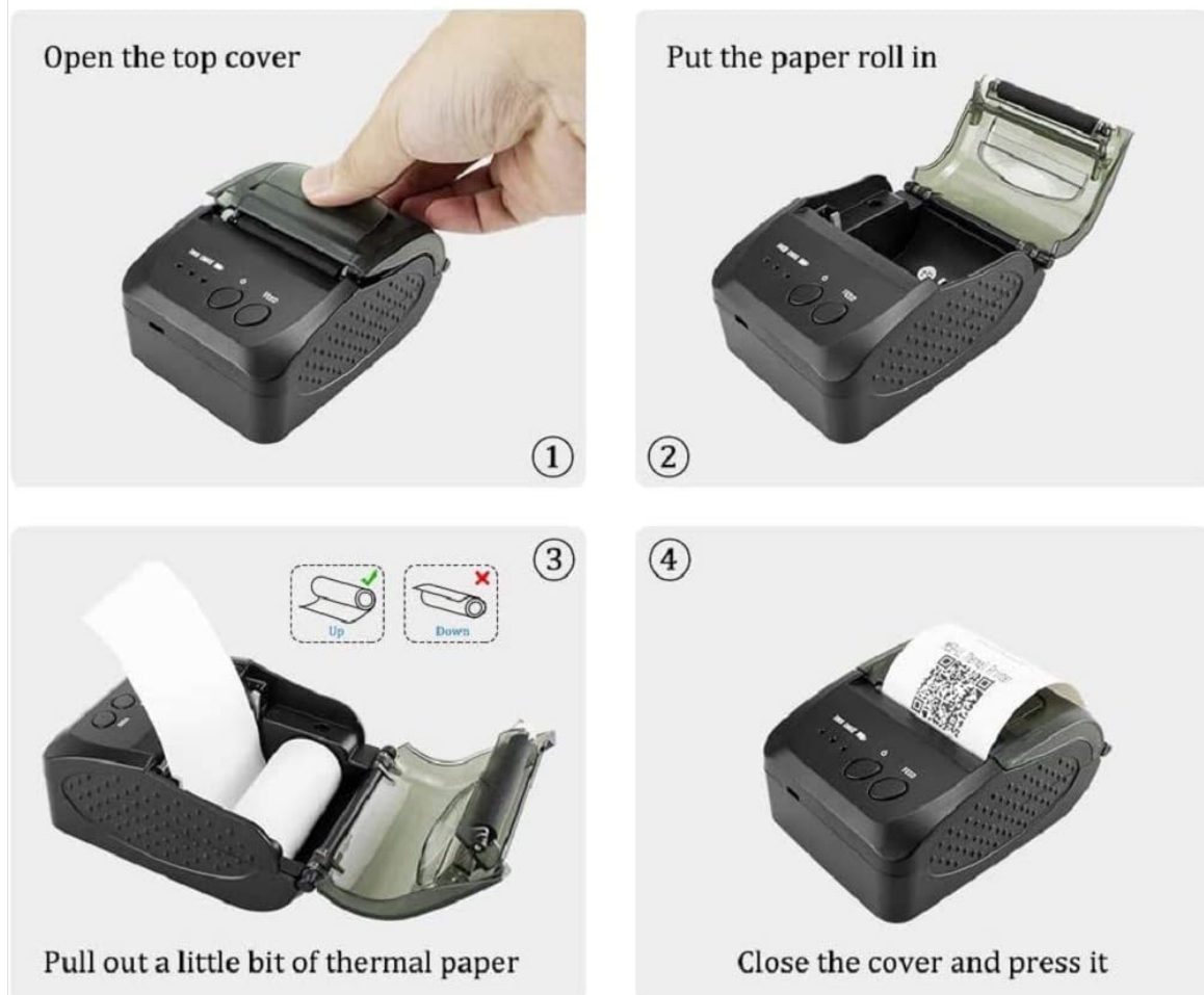
Figure 3.1: Step-by-step guide for loading thermal paper.
