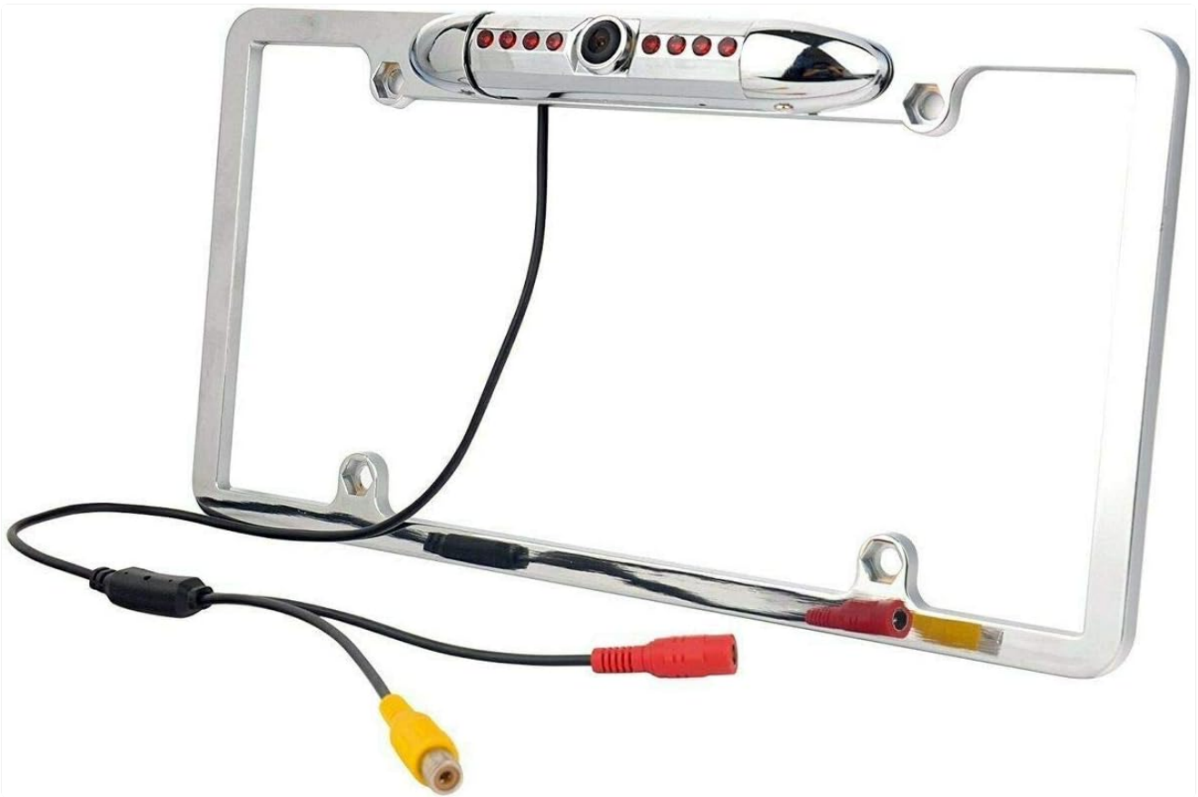
Figure 3.1: Absolute USA VZ-401 Night Vision Rear View Camera integrated into a chrome license plate frame. The camera unit is positioned at the top center of the frame, featuring a central lens flanked by multiple infrared (IR) LEDs on both sides for night vision capabilities. A black cable extends from the camera unit, leading to yellow and red RCA connectors for video and power connections, respectively. The chrome frame is designed to mount around a standard vehicle license plate.
