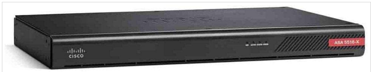
Figure 1: Front view of the Cisco ASA 5516-X Adaptive Security Appliance. This image displays the compact 1U rack-mountable chassis, featuring the Cisco logo on the left, status indicator lights (USB, Active, Status, Power) in the center, and a red label with "ASA 5516-X" on the right side of the vented panel.
