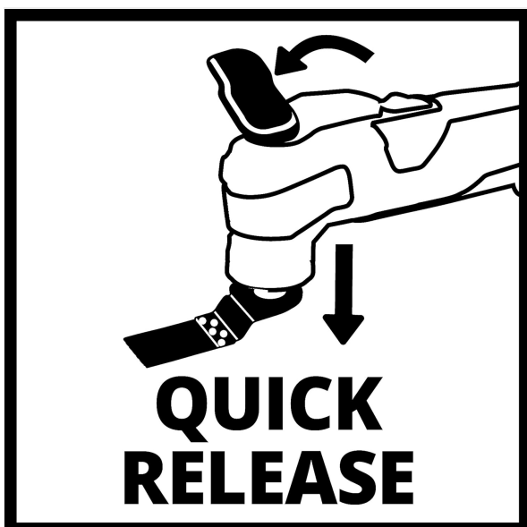
Figure 3.2: Demonstrating the attachment of an accessory blade to the multi-tool.
