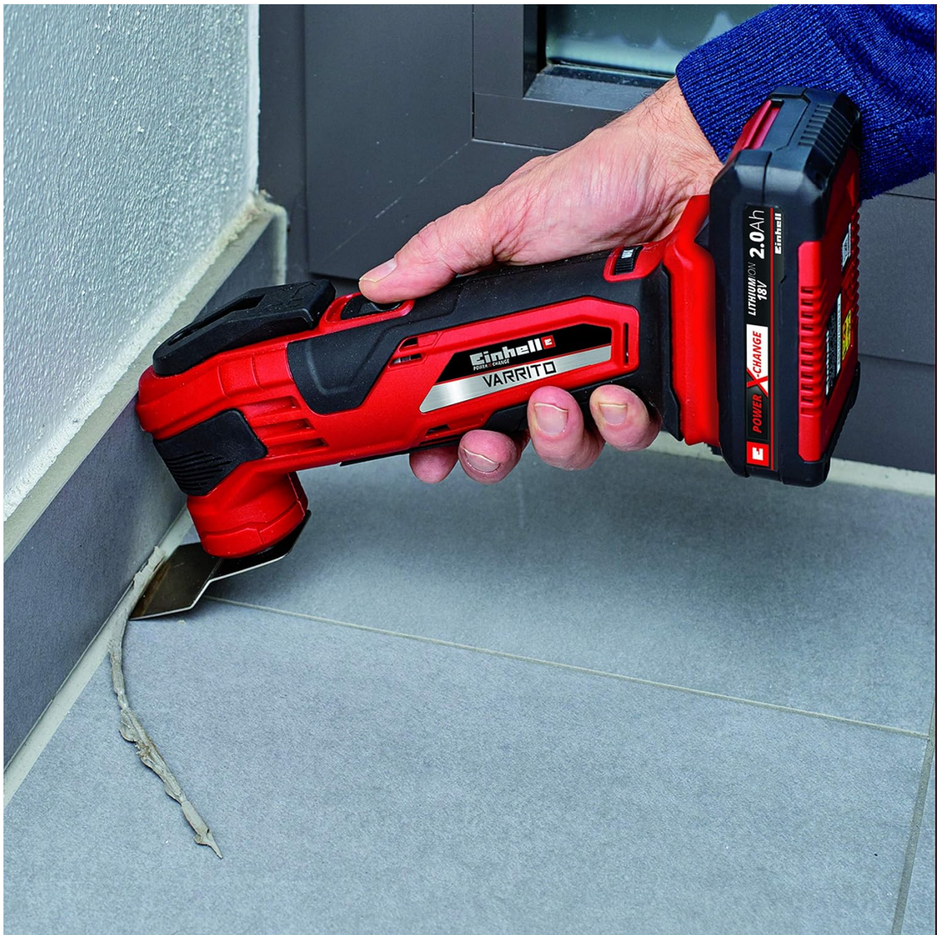
Figure 4.4: The multi-tool being used with a scraper blade to remove material from a floor edge.
