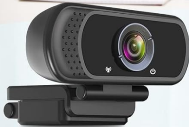
Image 5.2: The webcam's 110-degree wide-angle view, suitable for multiple participants.
